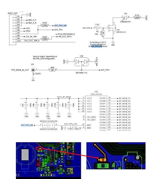
IRIGB at SMA with 50ohm load and 2.5V-fanout-driver-input, measured at **FCON\_1**. High level of 1.8V is achieved here, should be the same for FCON\_2.
