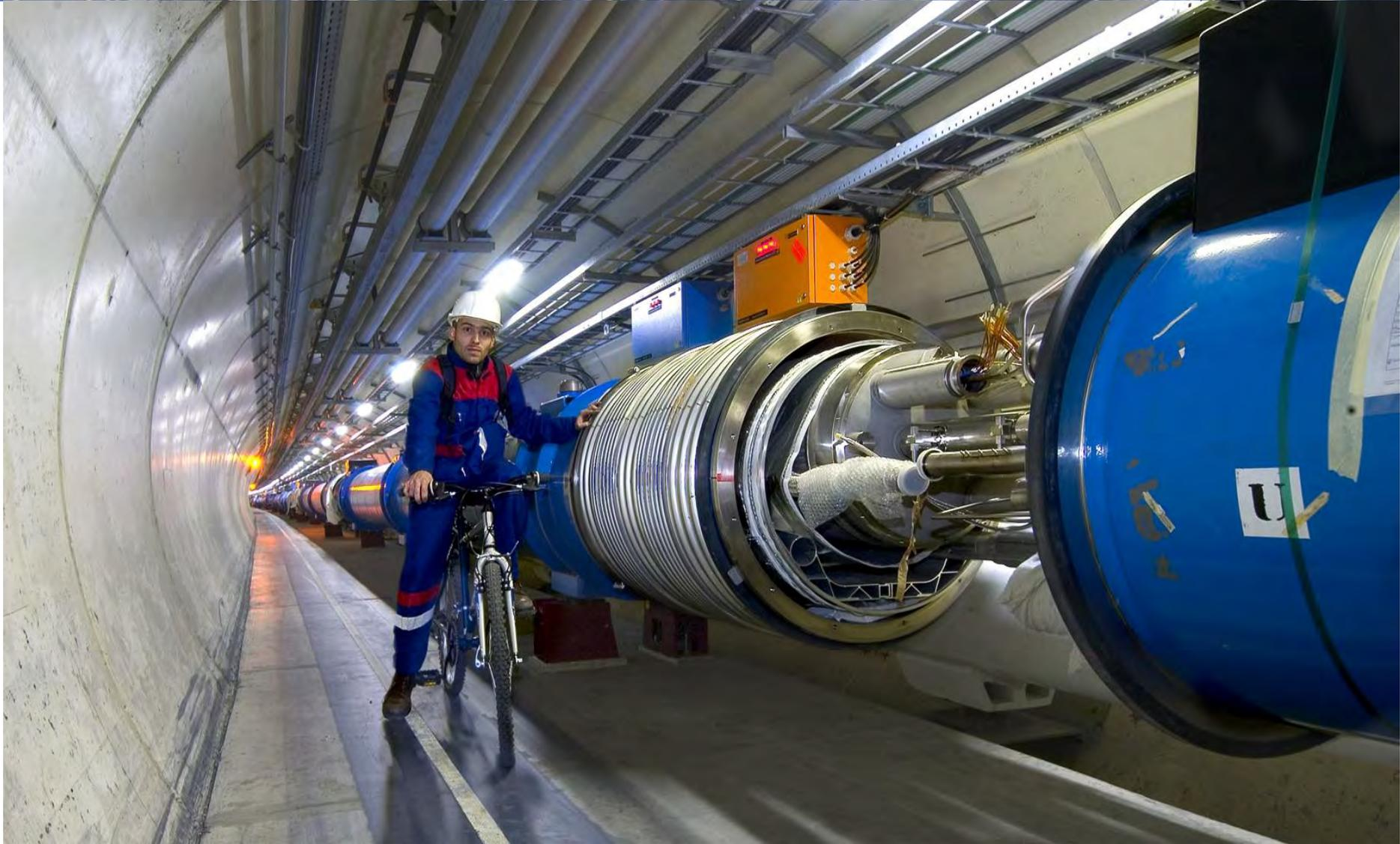
**$10^{14}$  protons in 2808 bunches circle the 27 km ring 11.245 times a second. The bunches cross 40 million times/s. Up to a billion protons/s interact.**
