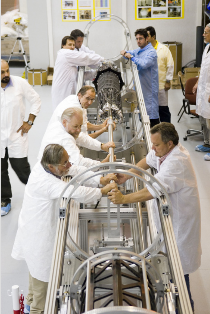
This month's photo is of the insertion of ATLAS pixel barrel layer 2 into the global support frame.
