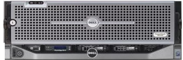
R610 + MD1000 JBOD Storage brick
