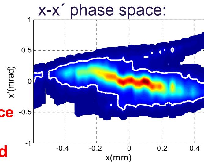
With a 10 % charge cut in the tails of the **phase space distribution** (~ remove non-lasing electrons)
