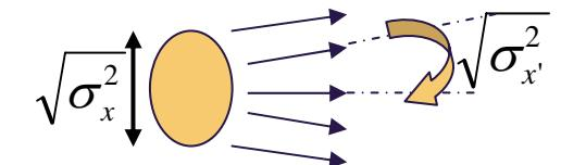
$\mathcal{E}$  = 6 dimensional phase space volume occupied by given # of particles
