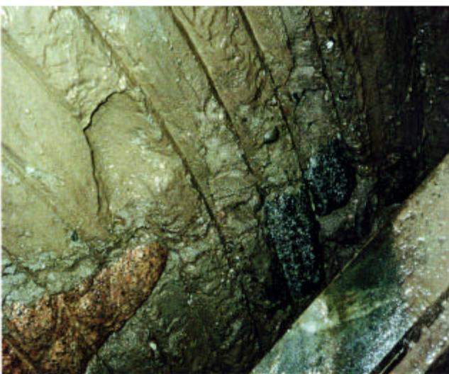
*Face with stones broken by disc cutters*
