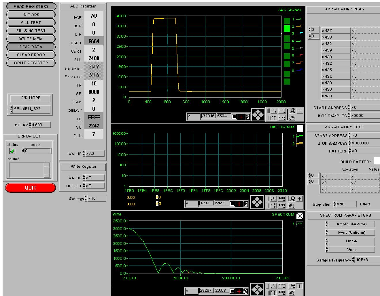
□ ADC test output for noise measurement (+/- 5V)
