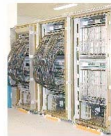
The APEmille computer racks at DESY Zeuthen. Each rack contains 100 nodes.
