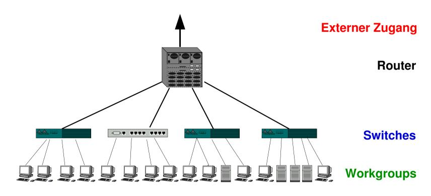
Using of Switches allows no central probe.
