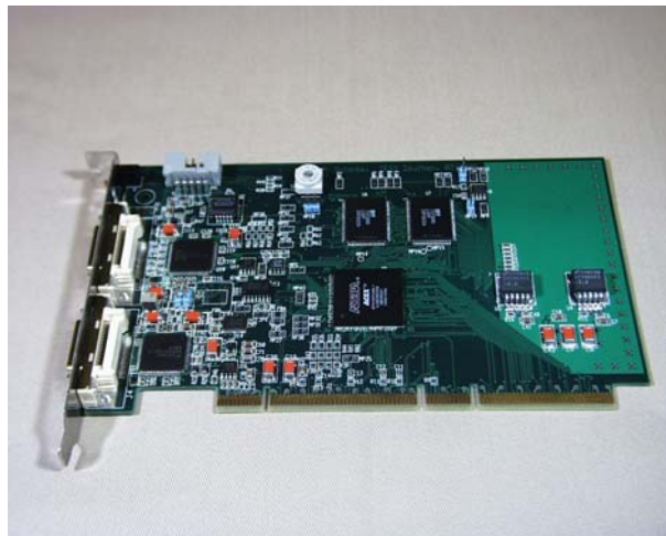
8 layer PCB, partial High Pad
