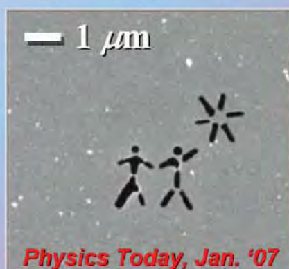
Starting Image (etched into silicon nitride film)
