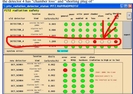
d. the detector 4 has "chamber loss" and "shorting plug of"
