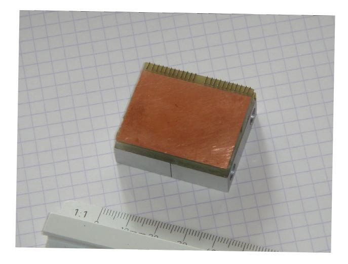
48 channels Strips made of AI foil have thickness corresponds to 0.75 μm Detector window is placed on front surface
