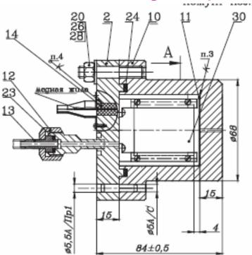
**Connector consists of covered capton foil with thickness of 100 micrometer**
