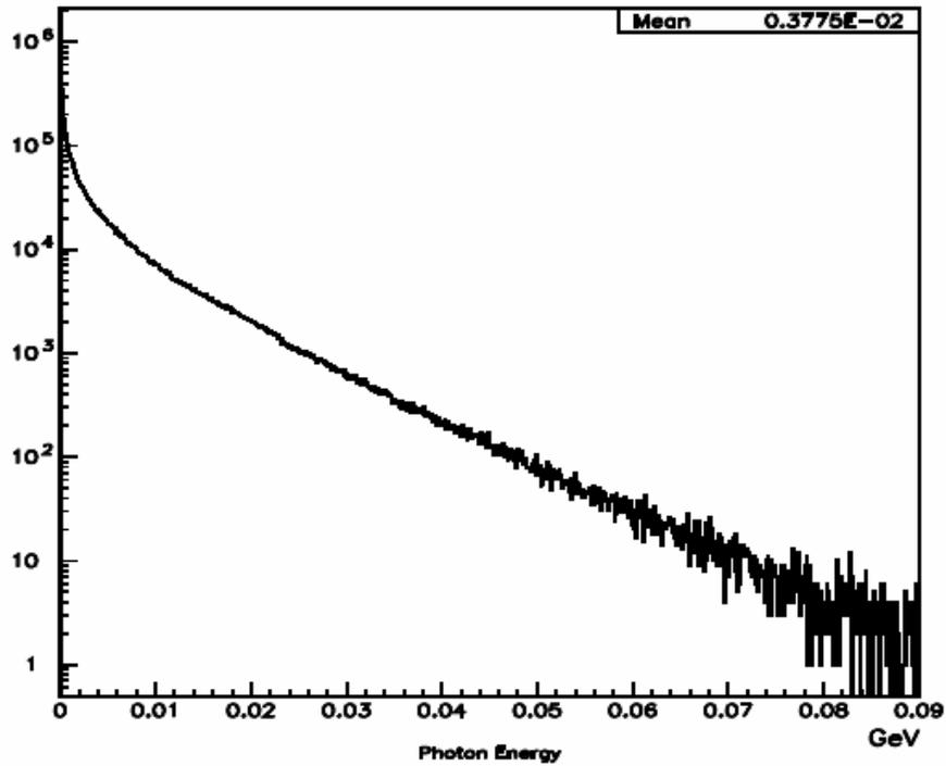
Energy of photons radiated within the spectrometer magnet.
