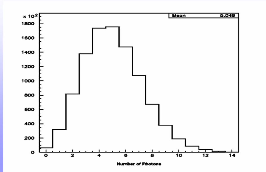
Multiplicity of photons radiated by an electron within spectrometer magnet, GEANT simulation
