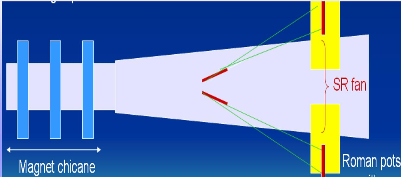
The application of mirrors permits to avoid the problems related to SR radiation protection however the installation of mirrors reduces the energy resolution at fixed coordinate resolution and detector position.
