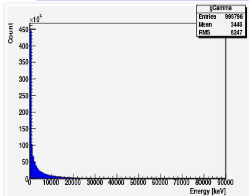
Energy of photons radiated within all 3 magnets.
