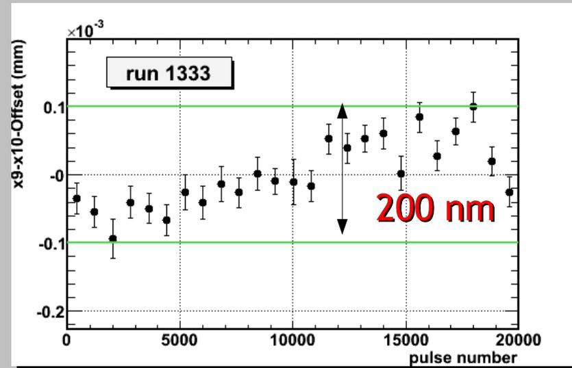
Resolution : BPM 3-5: ~ 700 nm in x, BPM 9-11: ~350 nm in x
