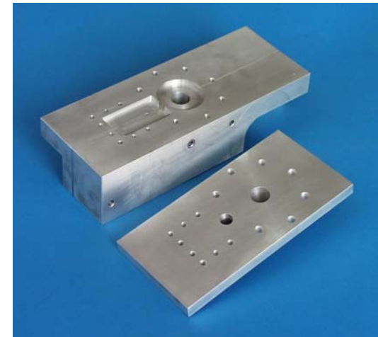
reference cavity disassembled
