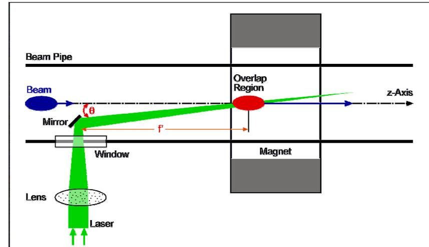
i.e. it is determined by the laser wavelength, so that for a given  $\lambda \rightarrow$  **minimum of laser spot size**
