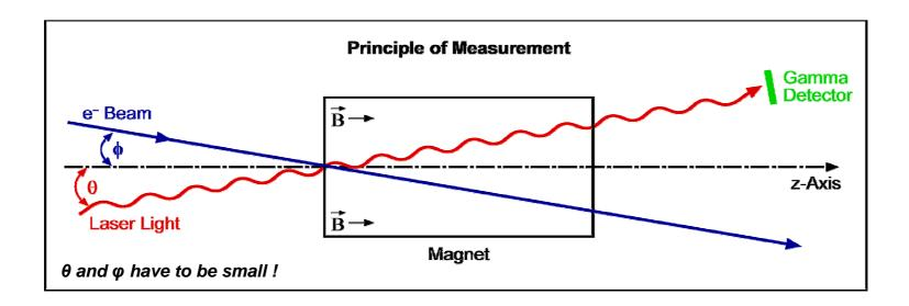
**RA** can be detected by measuring the ratio of the number of absorbed laser photons to the number of incident laser photons, i.e. the drop of the laser light intensity in the detector, as a function of a suitable quantity (e.g. the B-field) during the time of interaction of the beam particles with the laser light within the magnet.
