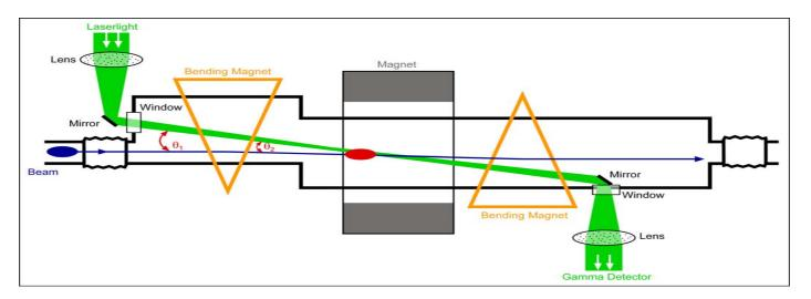
By changing the B-field in the first bending magnet,  $\varphi$  of the beam is changed, which in turn changes  $\theta$  ( $\theta_1 \rightarrow \theta_2$ ), the angle between the laser and the beam, by an amount  $\delta\theta$ .
