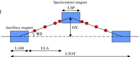
**O**= bending angle B= magnetic field 3 magnets (one analyzing, two ancillary) and a series of BPMs with high precision
