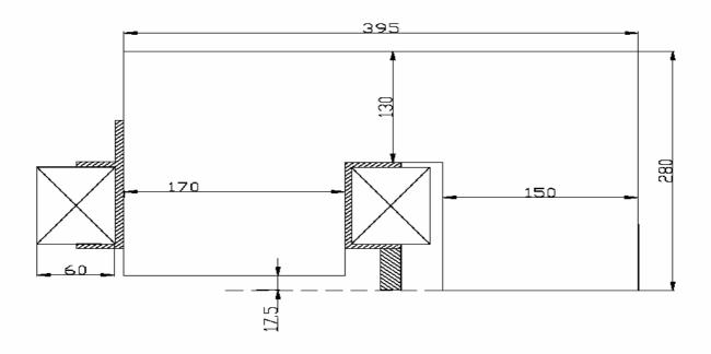
Basic technical parameters of the analyzing magnet.
