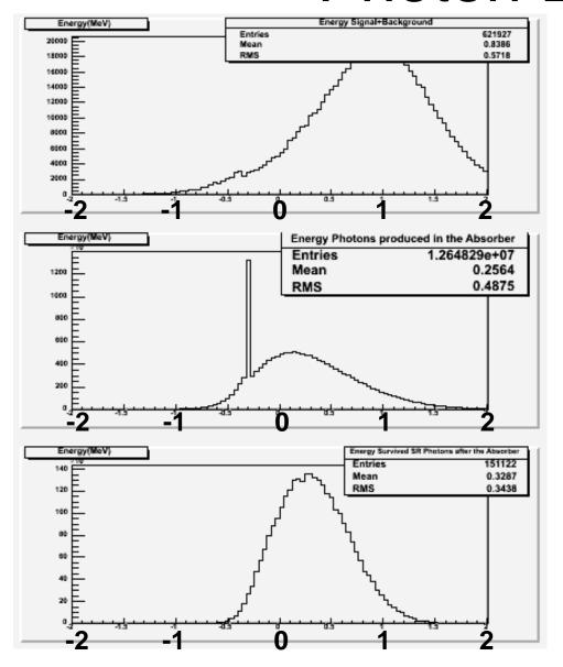
Energy Spectrum for charged particles produced in the absorber (**log(MeV)**)
