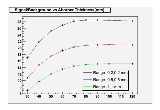
Plot made for lead (1 radiotion length 0.56 cm). Optimum is 60-80 mm (10-14 radiation length)
