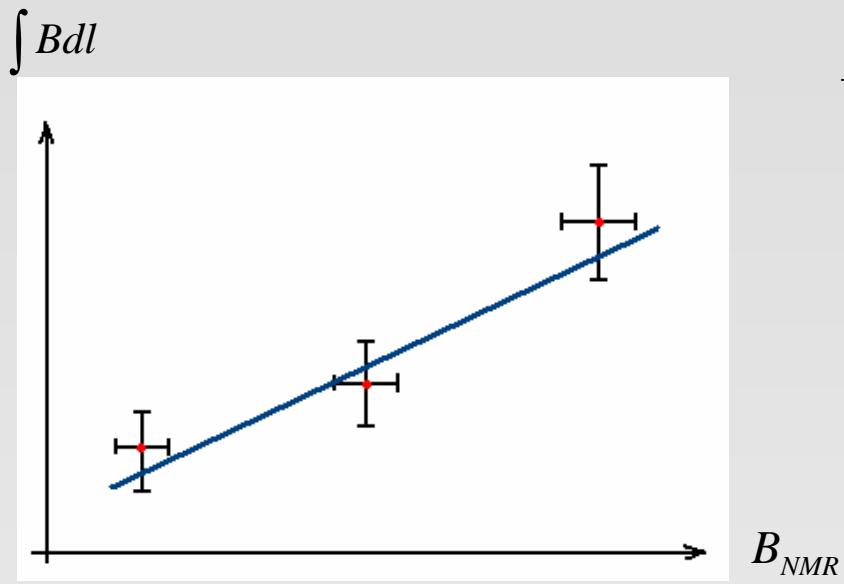
$$\frac{\Delta \int B dl}{\int B dl} = \sqrt{\left(\frac{\Delta B_{NMR}}{B_{NMR}}\right)^2 + \left(\frac{\Delta \int B dl}{\int B dl}_{meas}\right)^2 + \left(\frac{\Delta fit}{fit}\right)^2}$$
