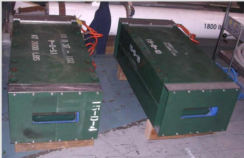
The distributions of the fringe residual magnetic field on the axis of the beam pipe outside the magnets 10D37 (#15-D-4 and #15-D-10) were measured
