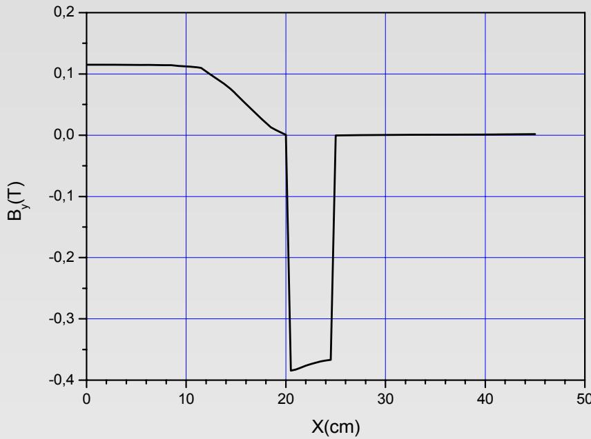
Magnetic field of the magnet in the middle transverse cross section
