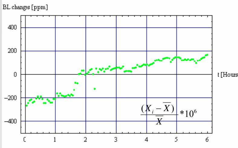
Magnetic field integral RMS stability ( $2\sigma$ ): **270 ppm**
