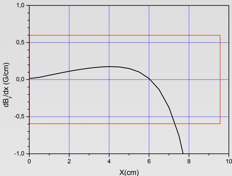
Magnetic field gradient in the middle cross-section of the magnet
