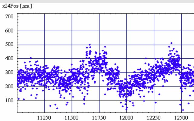
Resolution of the BPM4 in this run is about **3.4 microns**
