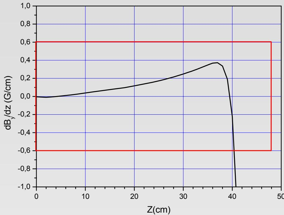
Magnetic field gradient in longitudinal direction
