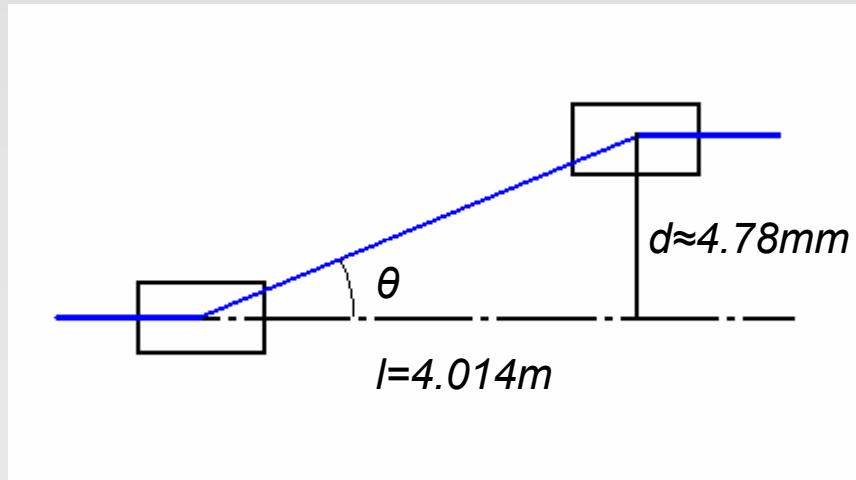
$$\theta = \arctg \frac{d}{l} = f(d) \quad |\Delta \theta| = \Delta d \cdot \frac{\partial f(d)}{\partial d}$$
