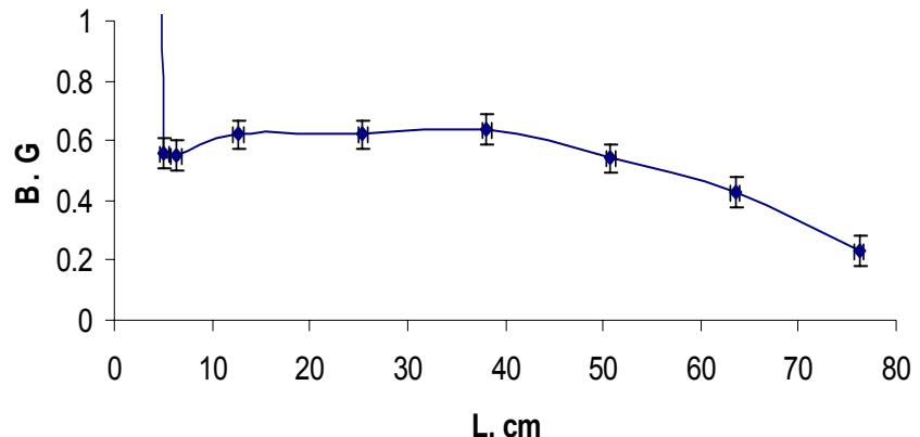
The residual fringe magnetic field of the magnet 10D37 #15-D-4
