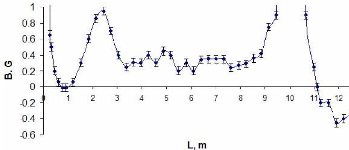
The anomaly behavior of the magnetic field on the distance near 10 meters is connected with the magnetic elements (impurity) in the girder.
