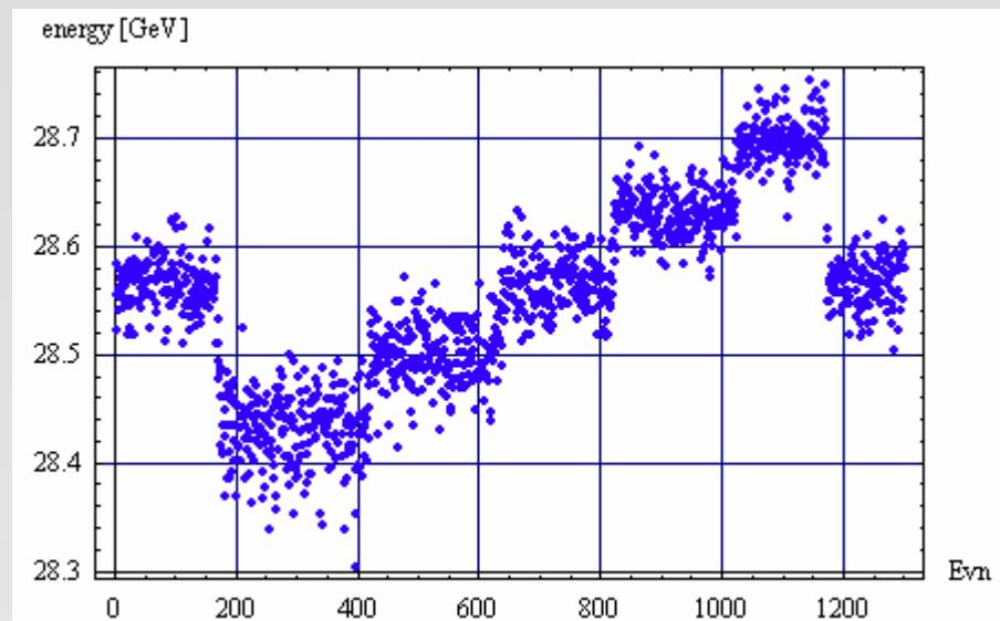
Run-1699: magnet scan with energy feedback setpoint at each setting
