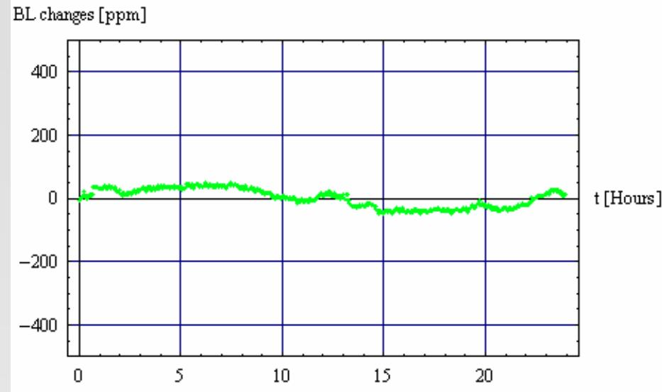
Power supply RMS stability ( $2\sigma$ ): **130 ppm**
