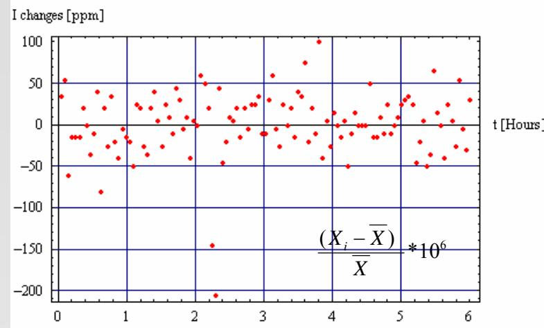
Power supply RMS stability ( $2\sigma$ ): **80 ppm**
