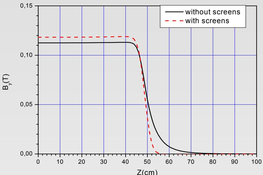
Magnetic field in the longitudinal direction
