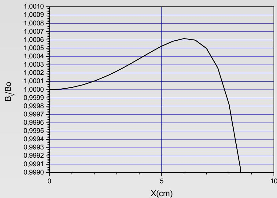
Normalized magnetic field in the middle cross-section of the magnet
