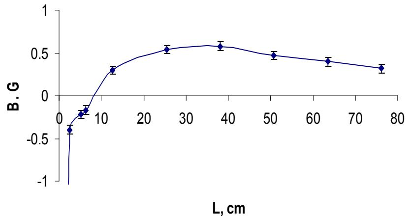
The residual fringe magnetic field of the magnet 10D37 #15-D-10
