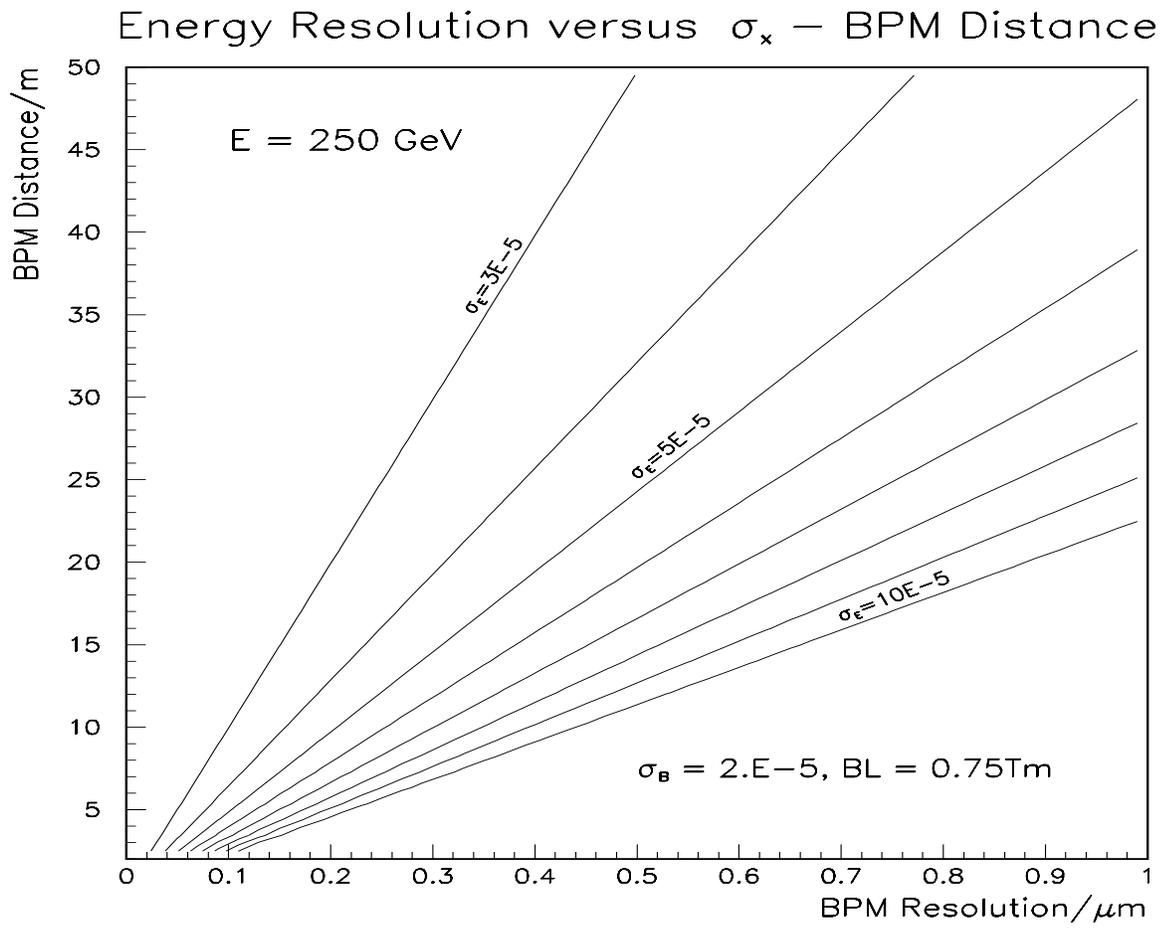
Figure 7: The lines of constant energy resolution in dependence on the BPM spatial resolution and the BPM distance.
