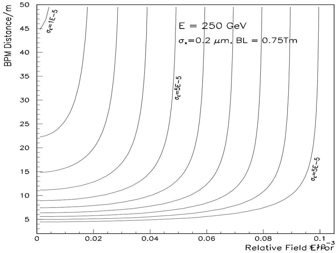
Figure 6: The lines of constant energy resolution in dependence on the relative field precision and the BPM distance.
