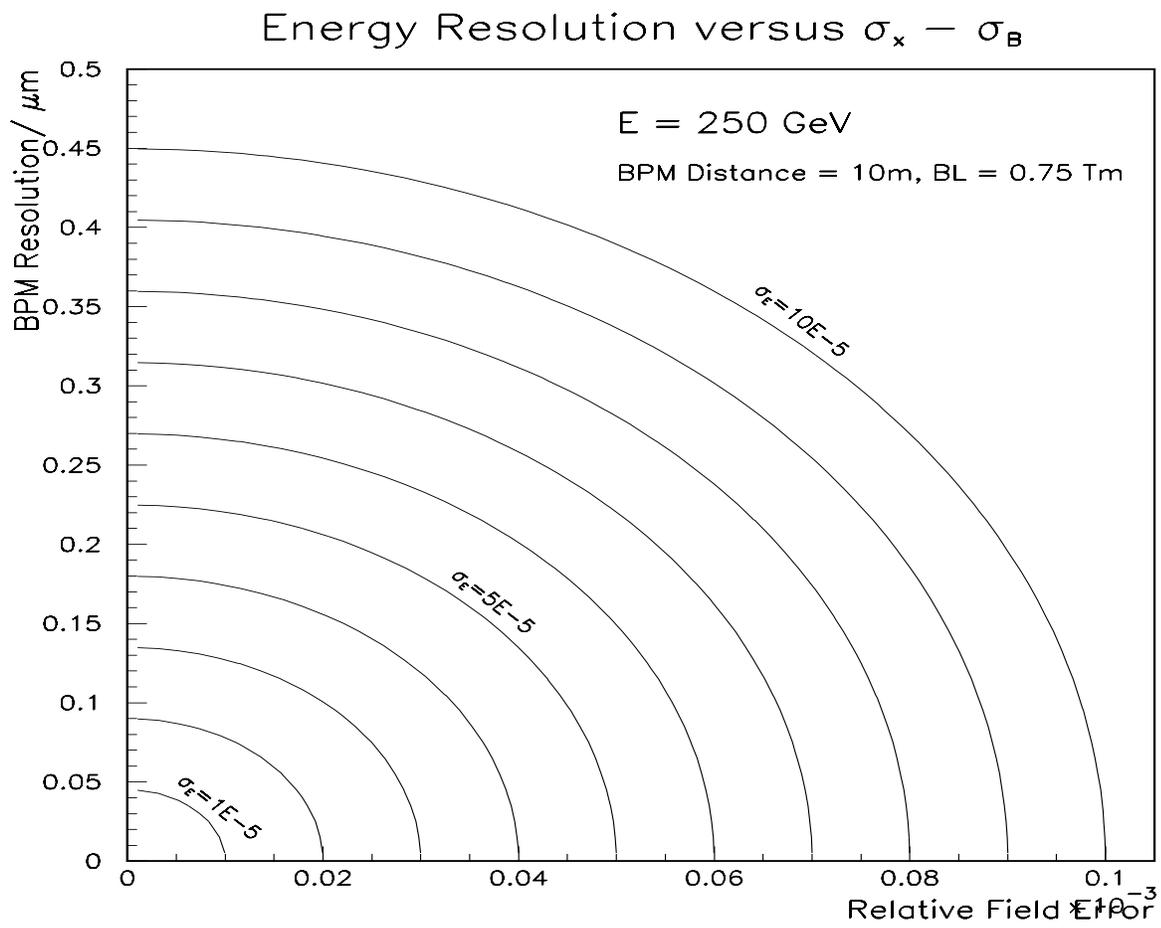
Figure 5: The lines of constant energy resolution in dependence on the relative field precision and the BPM spatial resolution.
