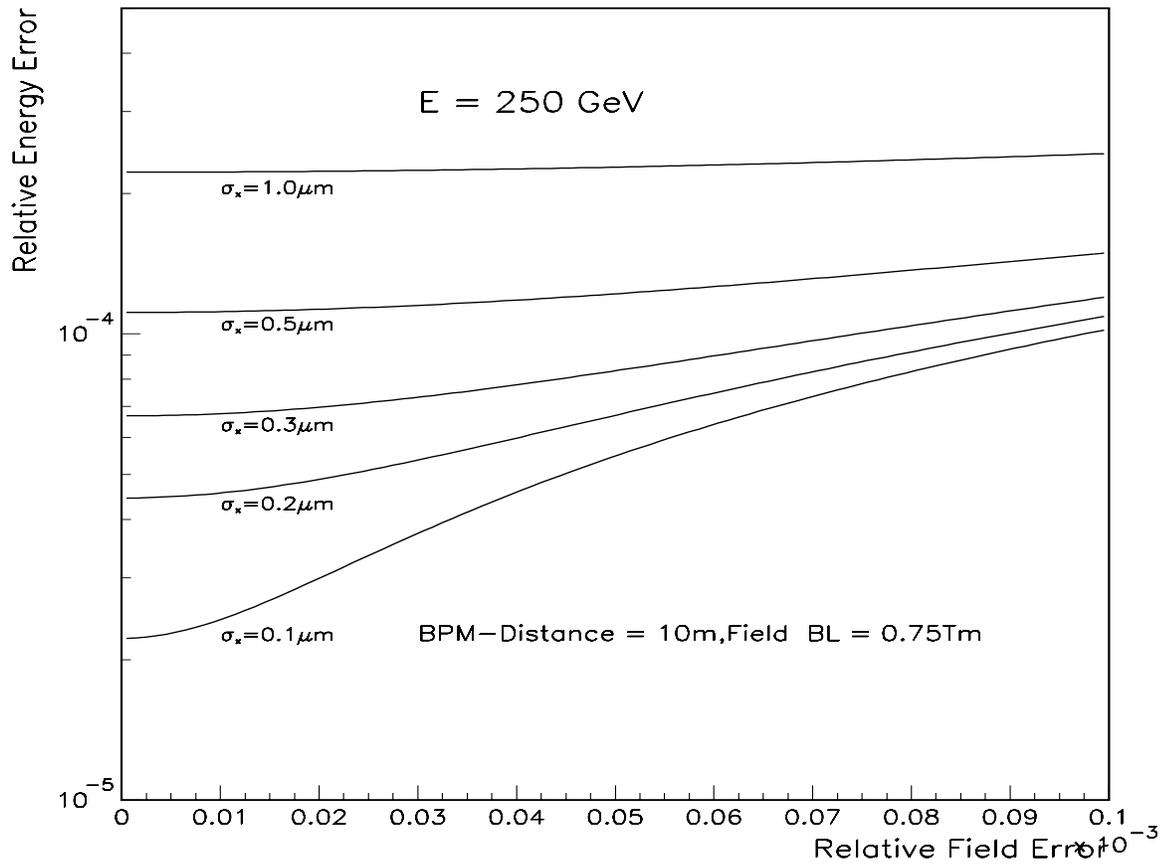
Figure 3: The energy resolution in dependence on the relative field precision. The lines describe different BPM spatial resolution.
