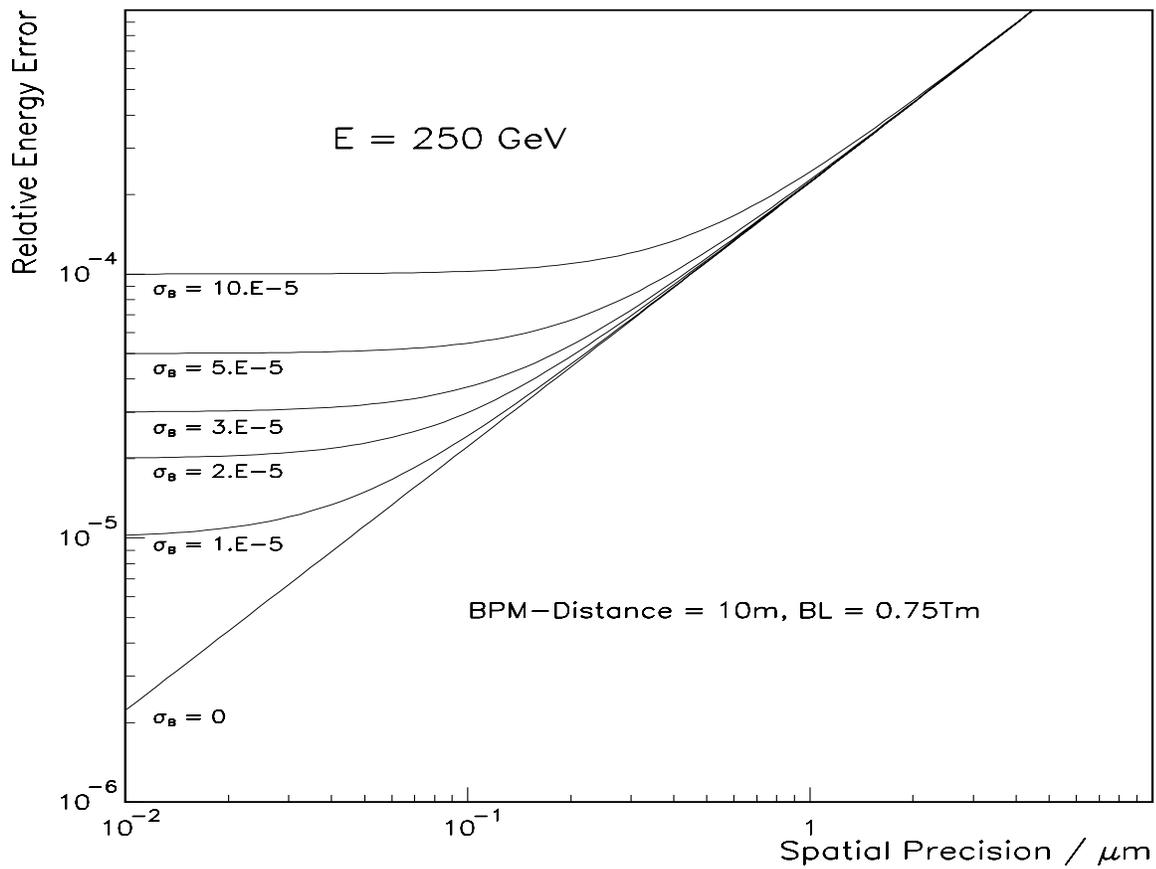
Figure 1: The energy resolution in dependence on the BPM spatial resolution. The lines describe different field precision in the range of a few  $10^{-5}$ .
