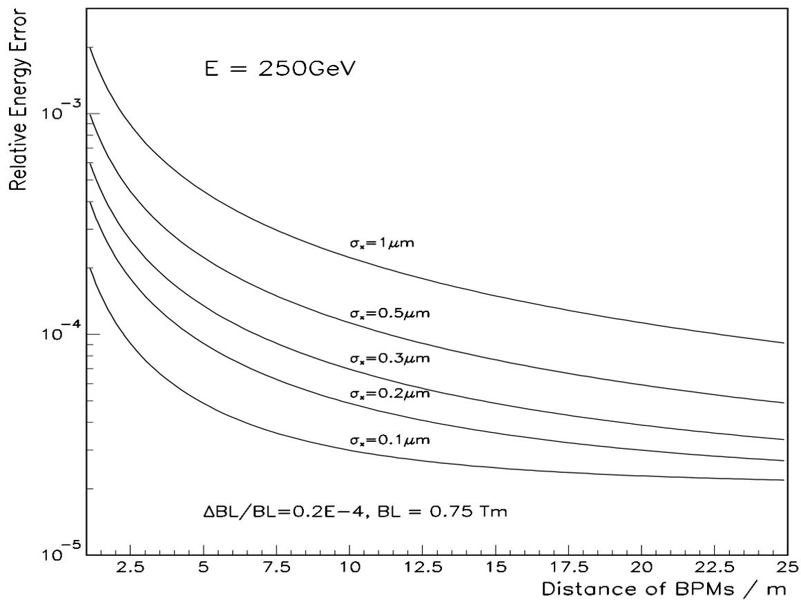
Figure 2: The energy resolution in dependence on the distance of the BPMs. The lines describe different BPM spatial resolution.
