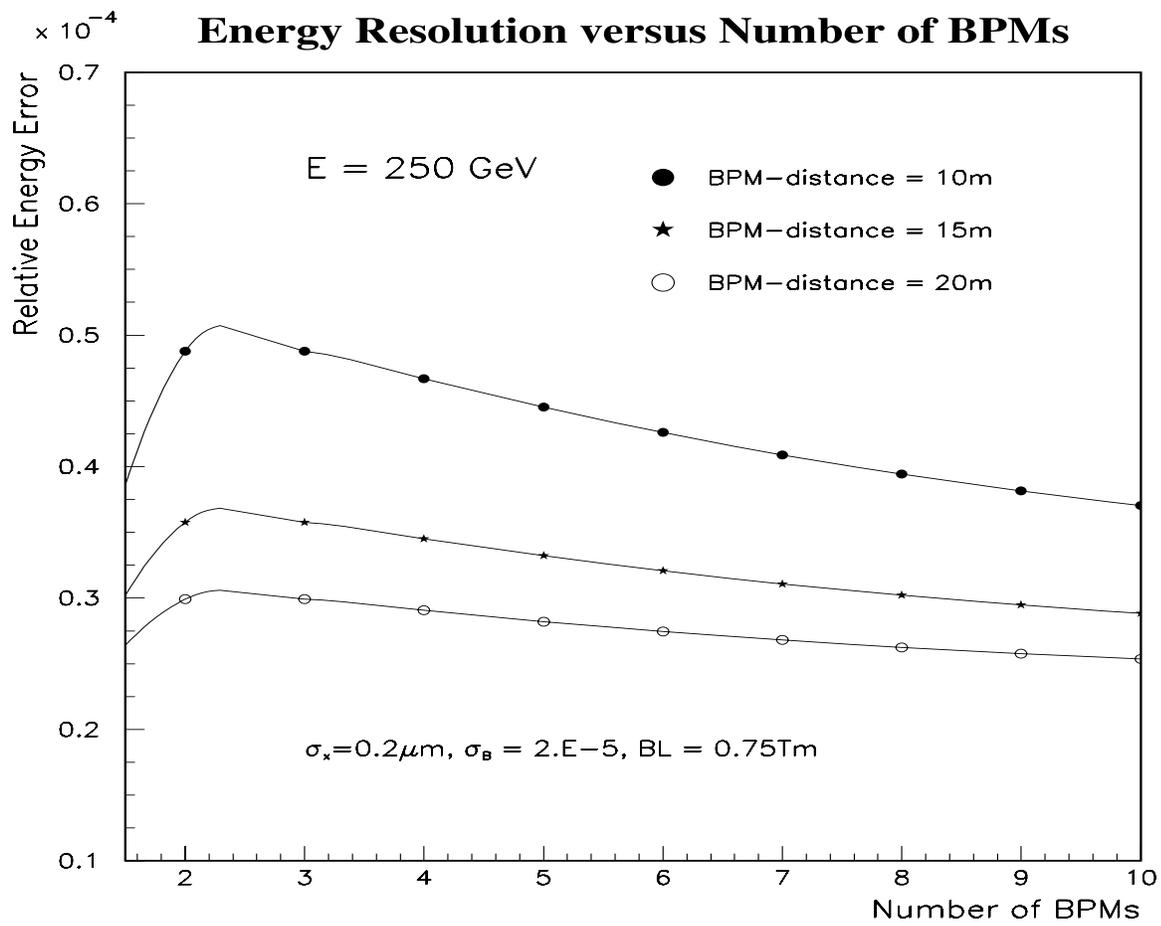
Figure 4: The energy resolution in dependence on the numbers of BPMs in each spectrometer arm. The lines describe different distances of the outermost BPMs.
