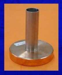
The vacuum prototype is made of copper. Some parts are made of stainless steel in order to achieve good vacuum properties. Most of parts are brazed together using hard-brazing.
