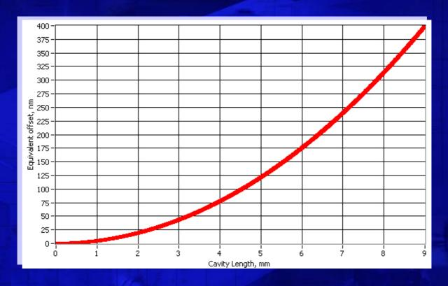
The incline component can be reduced by reducing the cavity length. The disadvantage – lower output signal.
