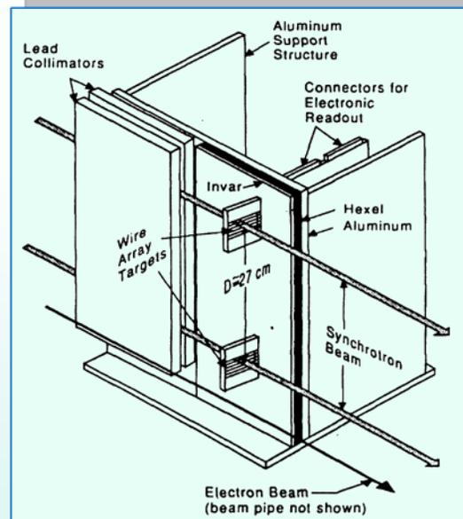
The SLC wire imaging synchrotron radiation detector
