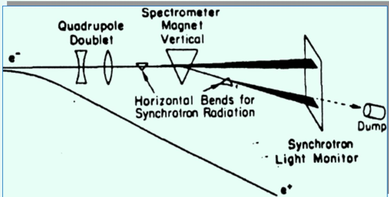
Conceptual design of the extraction-line SLC spectrometers
