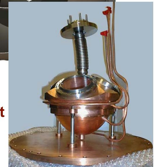
vacuum and target vessels (copper - low radioactivity)
