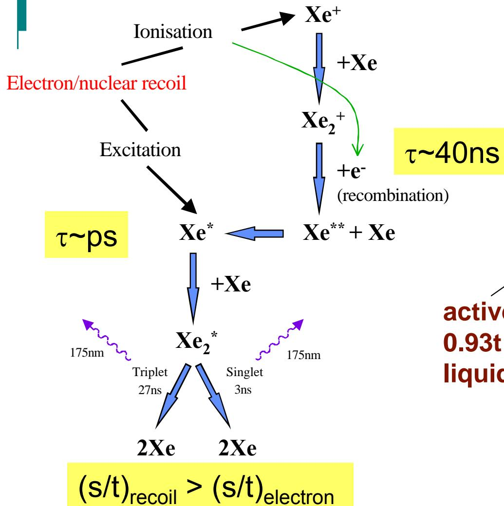
→ nuclear recoil pulses faster than electron recoils → PSD !
