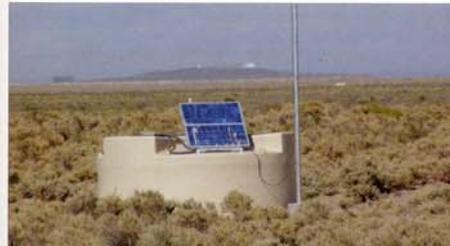
The Pierre Auger Observatory combines techniques used in earlier experiments to study cosmic-ray air showers at the highest energies. Water tanks, such as the one on the right, detect Cherenkov radiation produced by charged particles, while on dark nights optical detectors housed in larger buildings (left) record the faint light emitted as the showers cause fluorescence of atmospheric nitrogen. (Photos: Pierre Auger Laboratory.)
