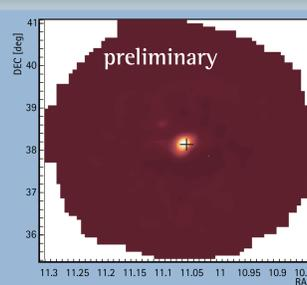
**MAGIC results.** In the left plot, the ALPHA distribution after cuts of the Mkn 421 simultaneous data set from 2004/12/18 (25 min) is shown. In the right figure, the sky map of reconstructed incoming direction of the gamma candidates for this data sample is presented. The sky map is smoothed using the angular resolution of 0.1°. The black cross indicates the actual position of the blazar Mkn 421.
