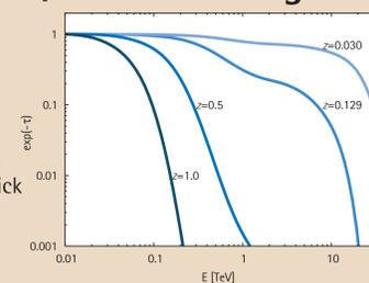
Attenuation factor exp(- $\tau$ ) for sources at four different redshifts:  $z=0.30$  (as Mkn 421, Mkn 501),  $z=0.129$  (as H1426),  $z=0.5$ , and  $z=1.0$  as a function of energy of GeV-TeV photons. The energy spectrum and the transition from optical thin to thick due to absorption on the extragalactic background light is well sampled by combined MAGIC/H.E.S.S. observations. The spectral distribution of the EBL is assumed as in [4]
