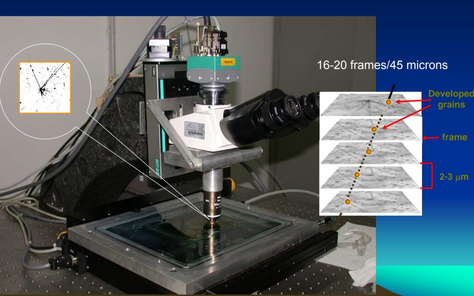
3D view of track segments reconstructed on both emulsion layers
