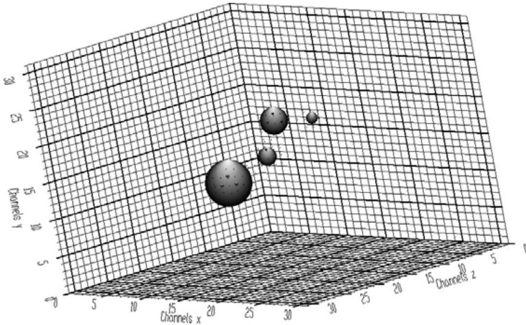
**Figure 20 Spectrum from Figure 19 after boosted one-fold Gold deconvolution (50 iterations repeated 20 times)**
