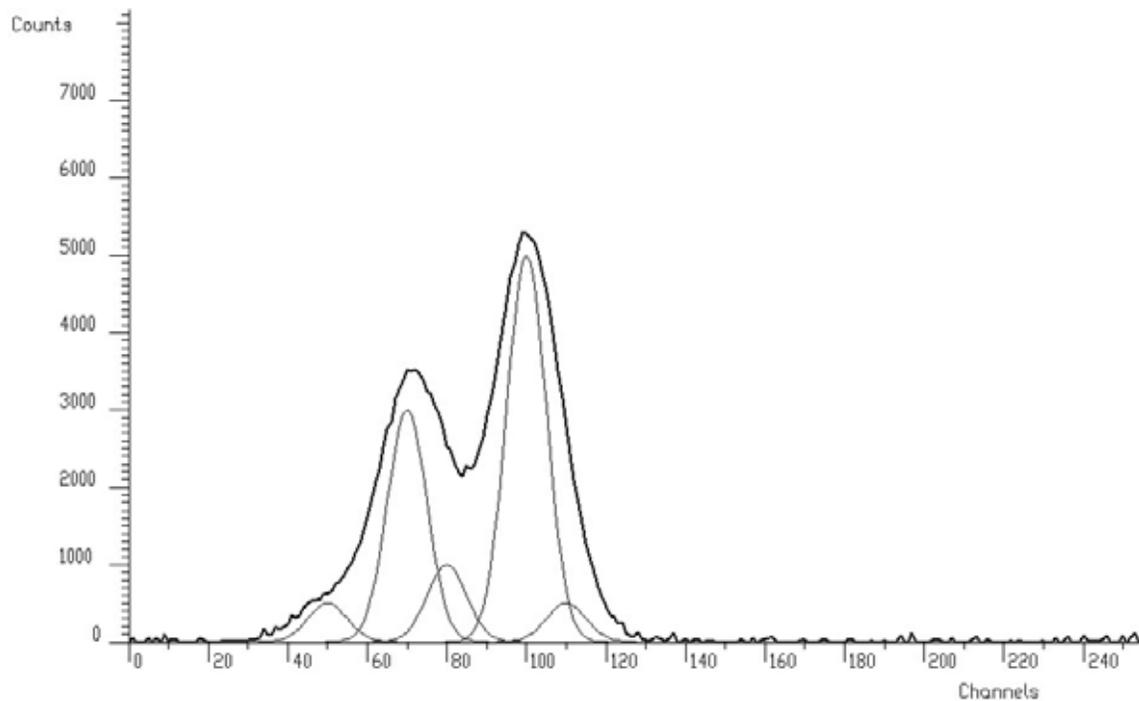
**Figure 25 Testing example of synthetic spectrum composed of 5 Gaussians with added noise**
