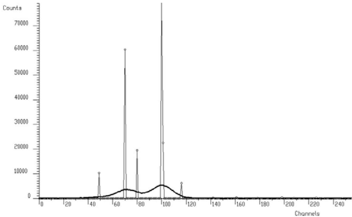
**Figure 41 Illustration of Muller algorithm of deconvolution with boosting**
