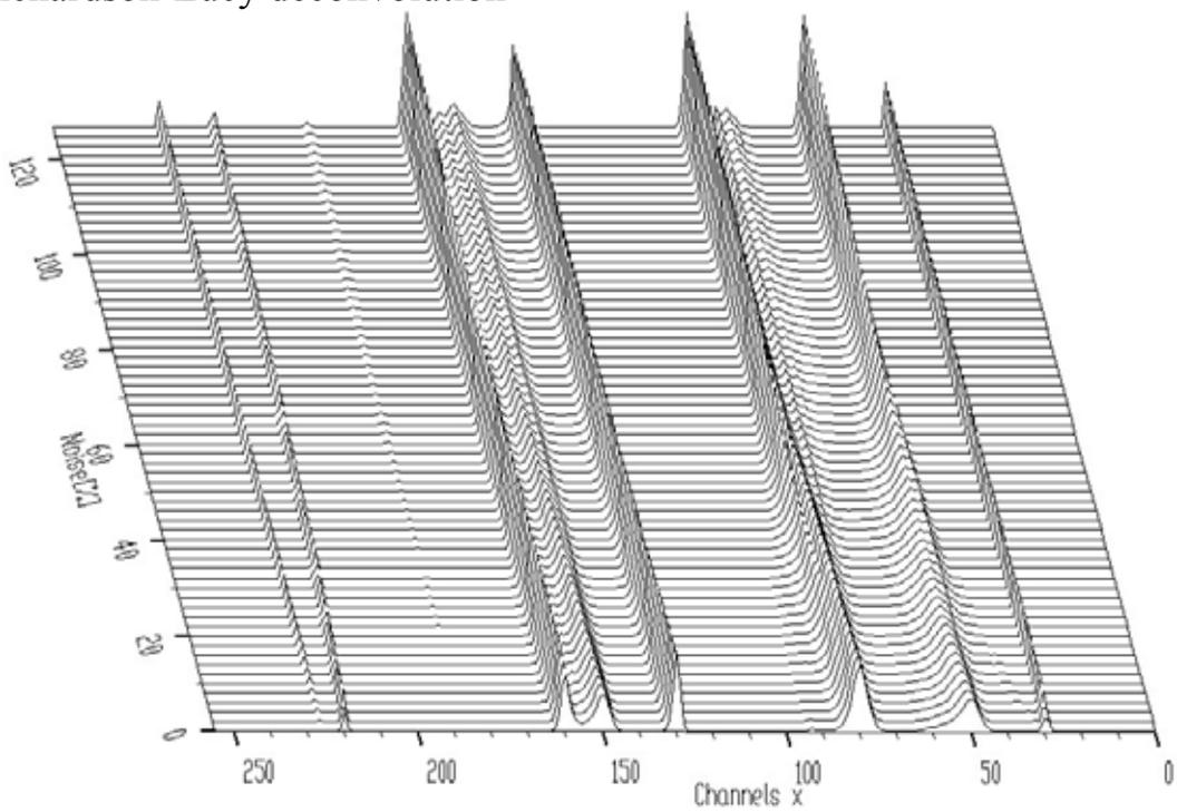
**Figure 48** Result of Richardson-Lucy deconvolution for increasing level of noise
