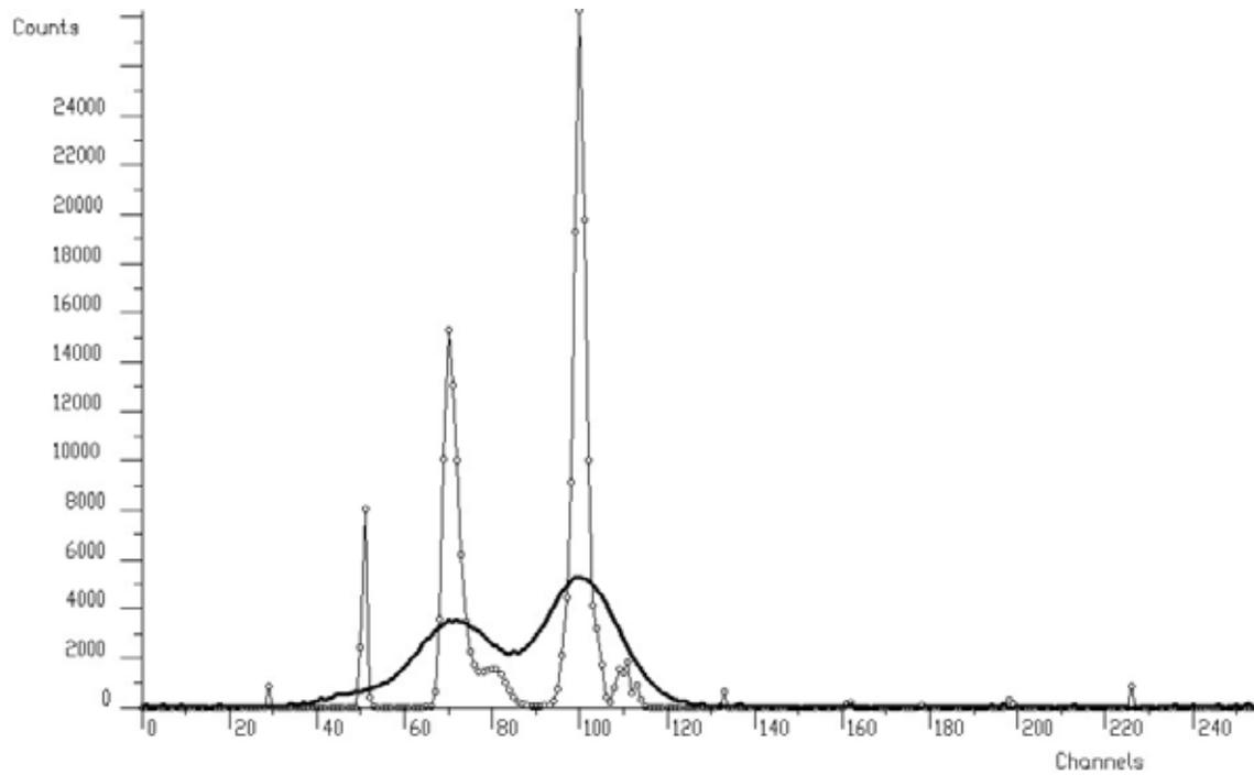
**Figure 38 Illustration of application of Richardson-Lucy algorithm of deconvolution**
