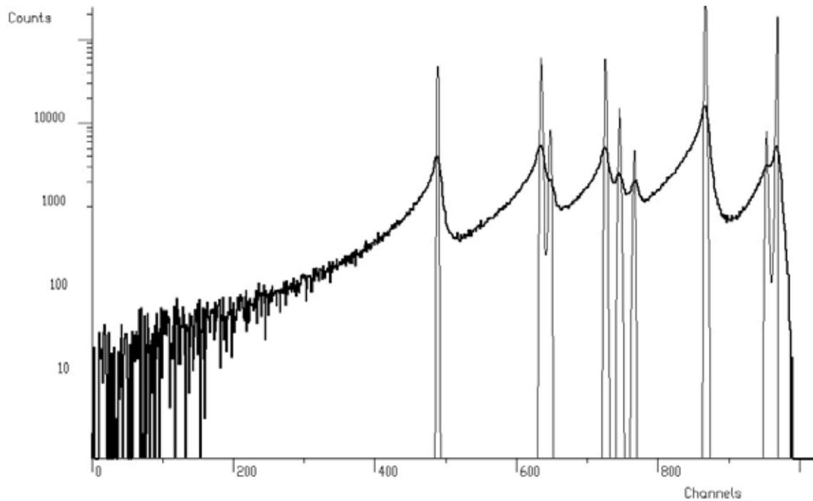
**Figure 23 Original electron spectrum (thick line) and deconvolved (boosted one-fold deconvolution - thin line)**
