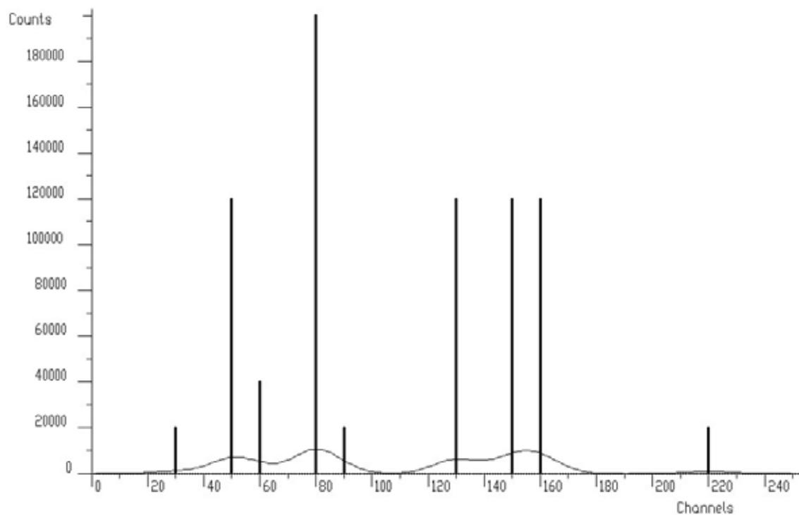
**Figure 2 Original (thin line) and deconvolved spectrum (bars) using unconstrained solution of Toeplitz system of linear equations**
