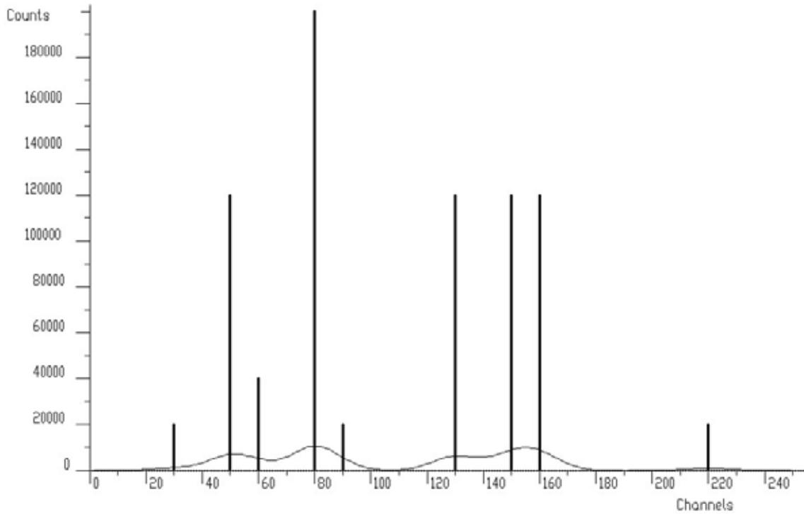
**Figure 43 Original synthetic spectrum (thin lines) and the ideal solution (thick bars)**
