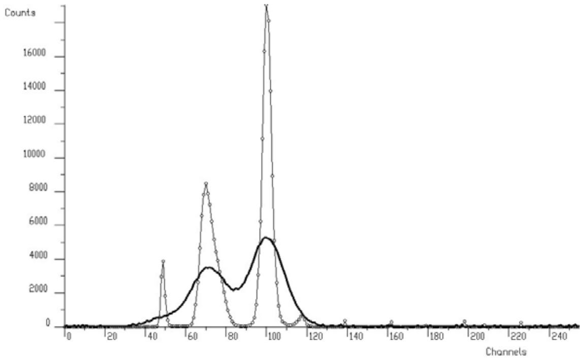
**Figure 40 Illustration of Muller algorithm of deconvolution**
