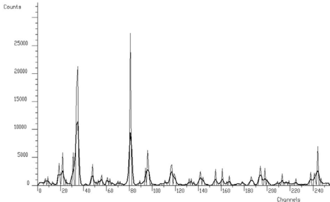
**Figure 11 Experimental  $\gamma$ -ray spectrum before (thick line) and after (thin line) boosted one-fold Gold deconvolution**
