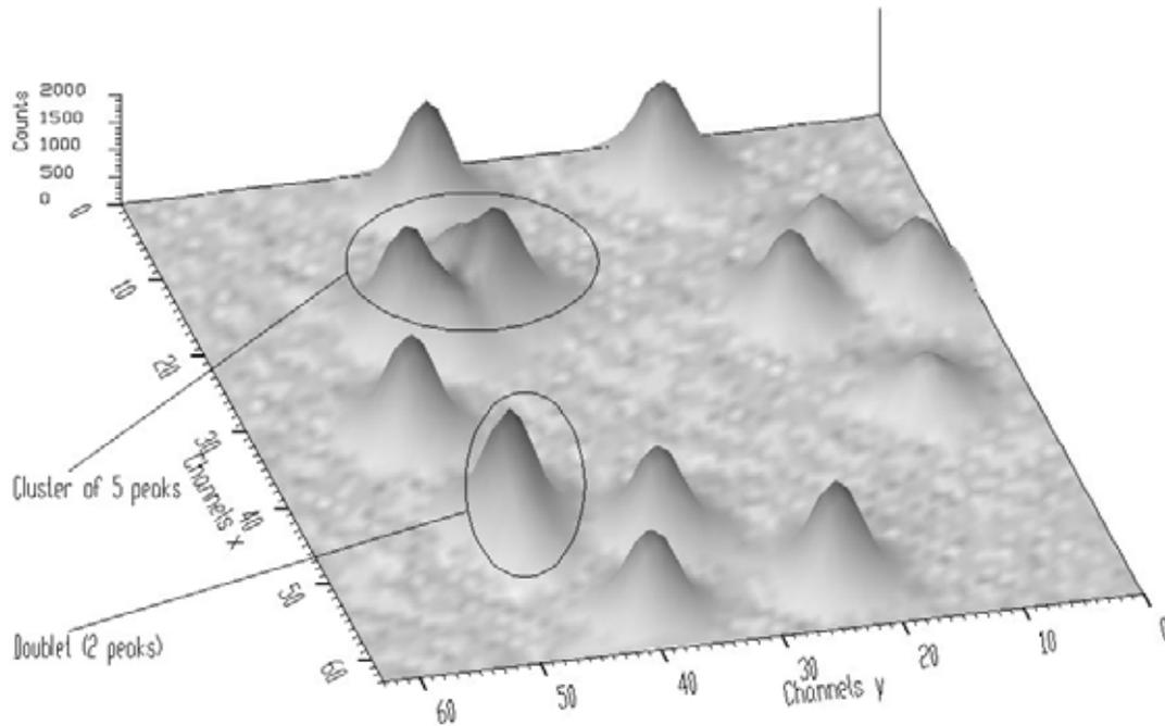
**Figure 12 Two-dimensional original synthetic spectrum**
