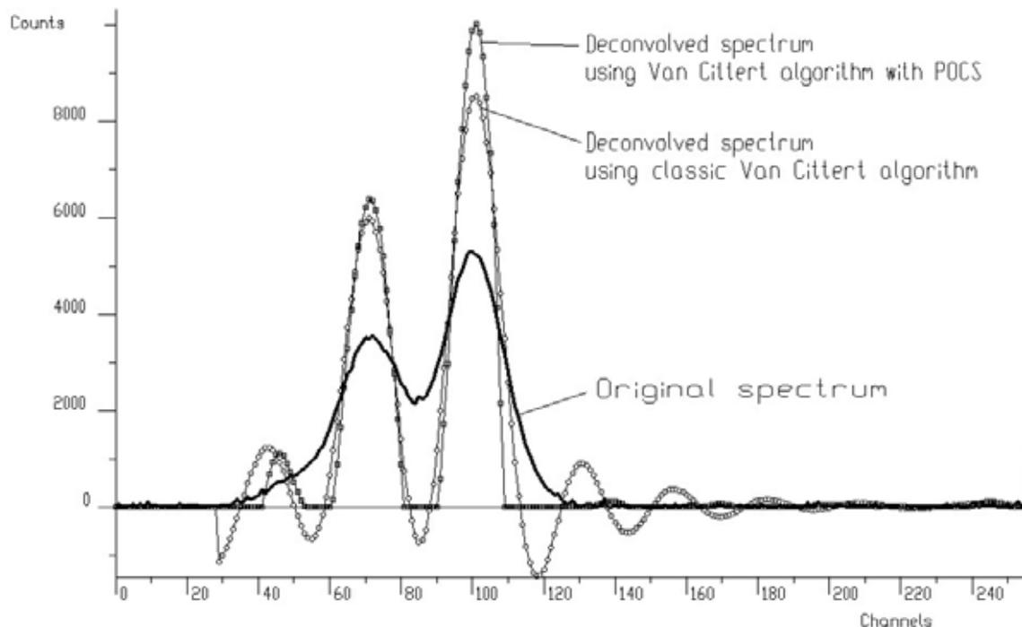
**Figure 35 Original spectrum (thick line), deconvolved using Van Cittert algorithm (without regularization) and deconvolved using Van Cittert algorithm and regularized via POCS method**
