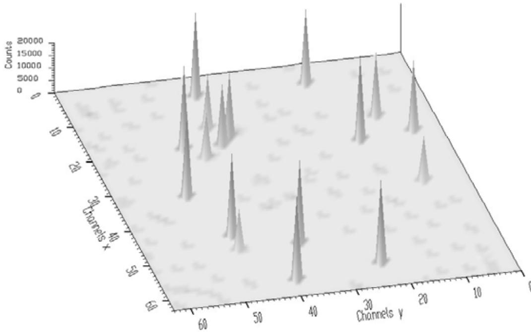
**Figure 15 Spectrum from Figure 12 after boosted one-fold Gold deconvolution (50 iterations repeated 20 times)**
