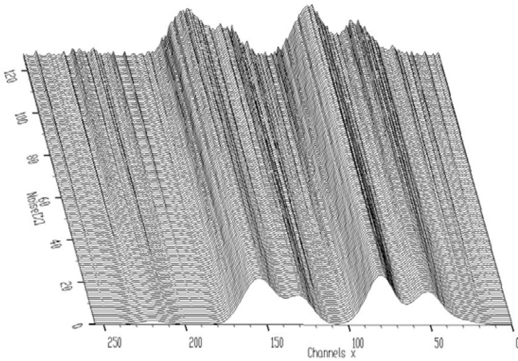
**Figure 44 Original spectrum with increasing added noise (in % of the amplitude of smallest peak in the spectrum)**
