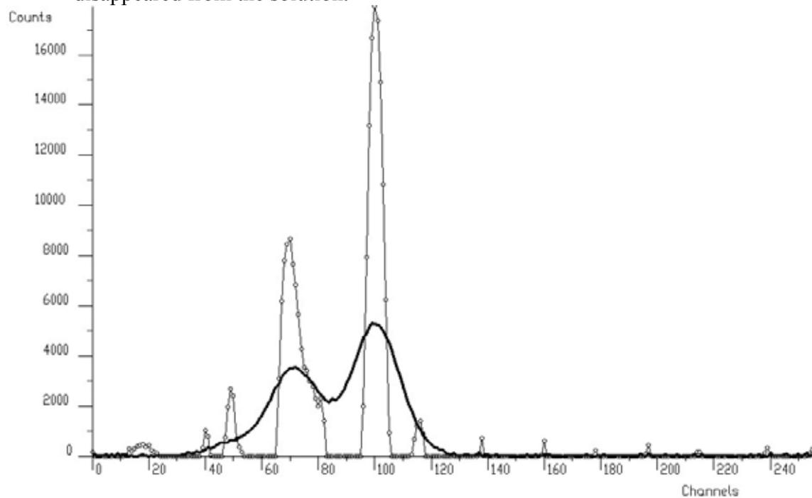
**Figure 31 Riley deconvolution with POCS regularization**
