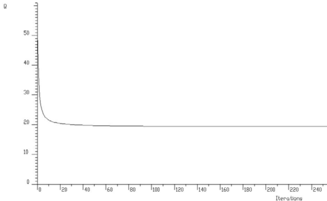
**Figure 8 Sum of weighted squares of errors per one channel in dependence on number of iterations**
