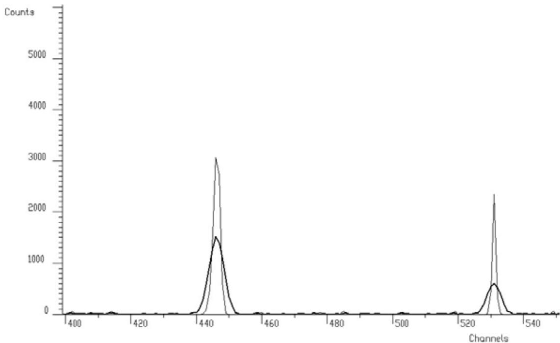
**Figure 6 Detail of the spectrum from Figure 5 (thick line) and after (thin line) two-fold Gold deconvolution (10000 iterations)**
