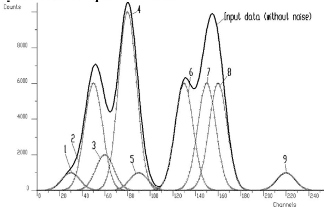
Figure 1 Example of synthetic spectrum (without noise) composed of 9 Gaussians
