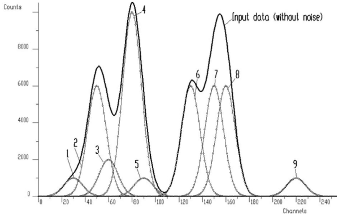
**Figure 42 Original spectrum composed of 9 Gaussians**
