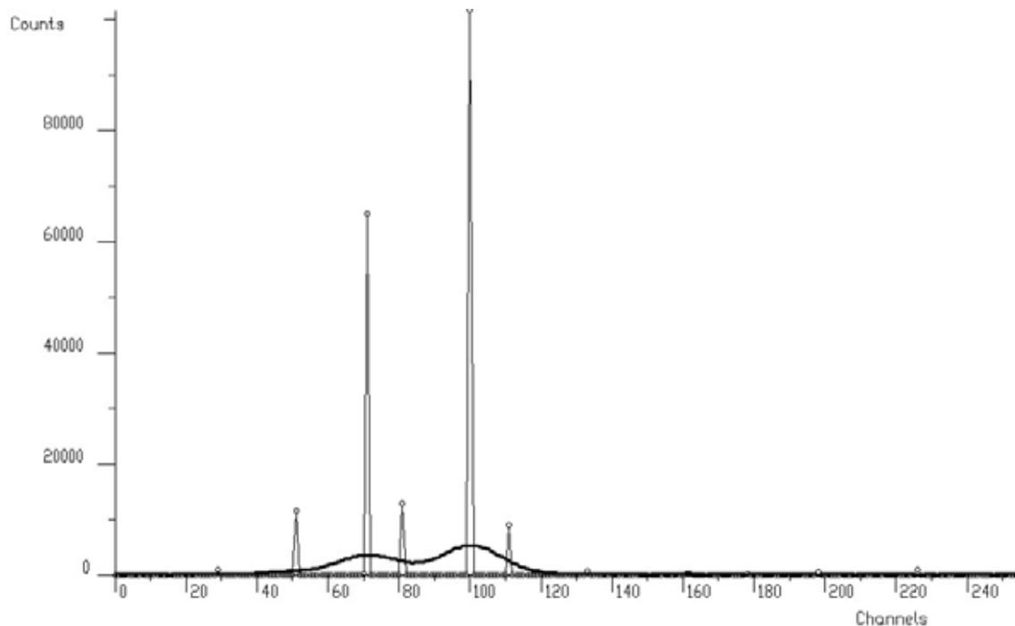
**Figure 39 Spectrum deconvolved using boosted Richardson-Lucy algorithm of deconvolution**
