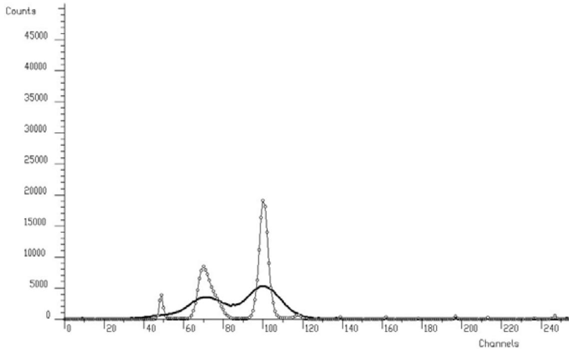
**Figure 36 Original spectrum (thick line) and deconvolved spectrum using one-fold Gold algorithm ( 10000 iterations, thin line)**
