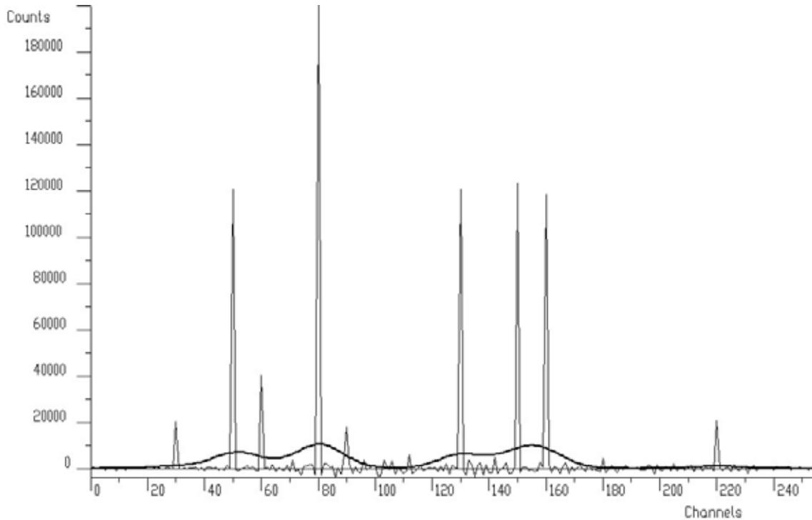
**Figure 4 Original spectrum from Figure 1 + channel 80 increased by one (thick line) and deconvolved spectrum (thin line) using unconstrained solution of Toeplitz system of system of linear equations**
