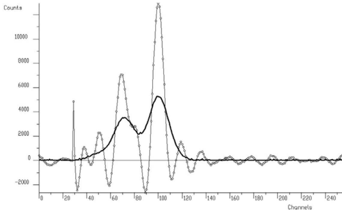
**Figure 30 Illustration of Riley algorithm of deconvolution**
