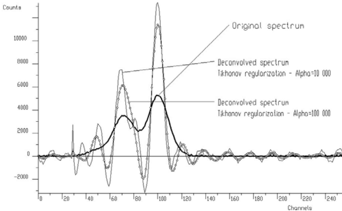
**Figure 28 Solution obtained using Tikhonov method of regularization**
