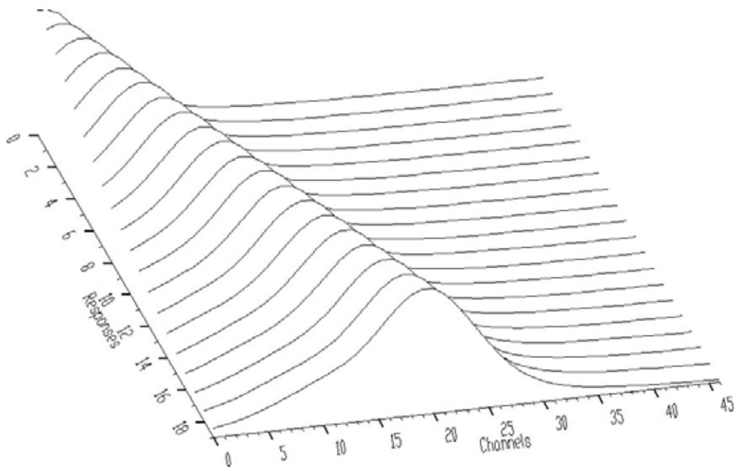
**Figure 22 Part of response matrix composed of response electron spectra**
