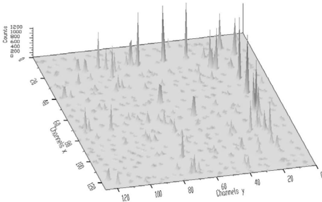
**Figure 18 Spectrum from Figure 17 after boosted one-fold deconvolution (50 iterations repeated 20 times)**
