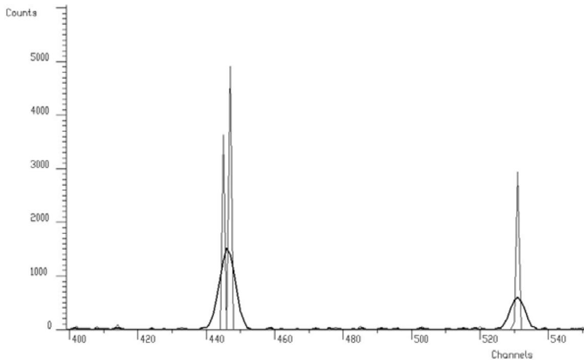
**Figure 9 Detail of the spectrum from Figure 5 before (thick line) and after boosted one-fold Gold deconvolution (shown in polyline display mode - thin line)**
