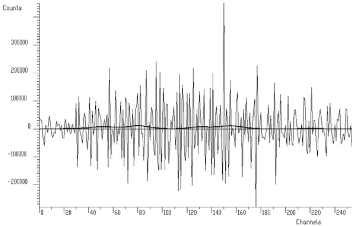
**Figure 3 Original spectrum from Figure 1 + 1% of noise of the smallest peak # 9 (thick line) and deconvolved spectrum (strong oscillations) using unconstrained of Toeplitz system of system of linear equations**
