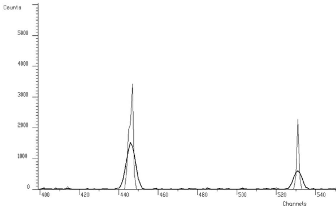
**Figure 7 Detail of the spectrum from Figure 5 before (thick line) and after (thin line) one-fold Gold deconvolutions (10000 iterations)**
