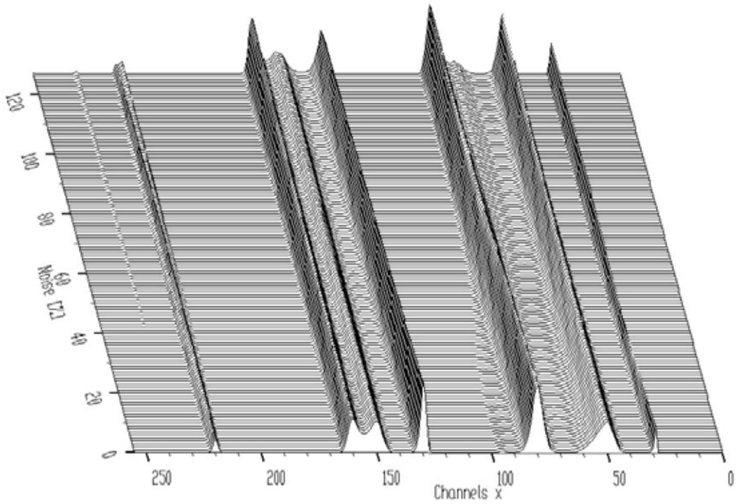
**Figure 46** Result of one-fold Gold deconvolution for increasing level of noise
