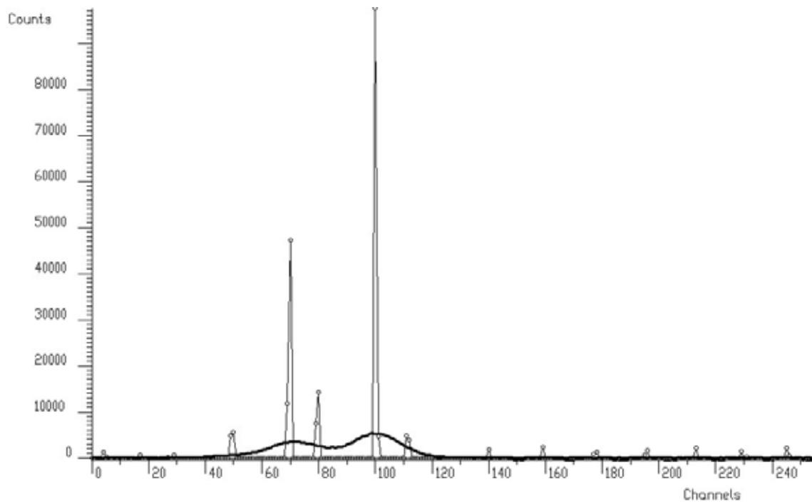
**Figure 33 New algorithm of deconvolution with minimization of squares of negative values (100 iteration steps)**
