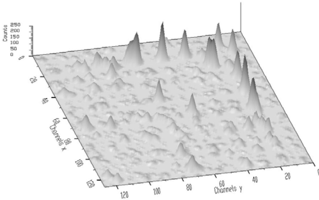
**Figure 17 Part of original experimental two-dimensional  $\gamma - \gamma$  coincidence spectrum**
