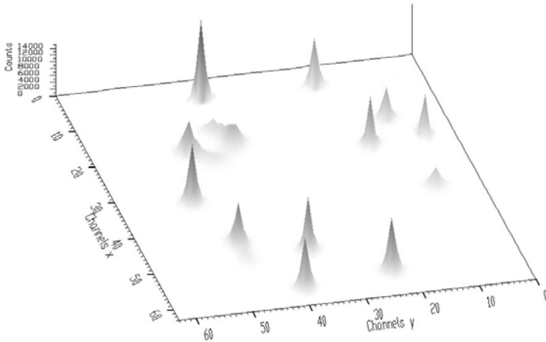
**Figure 13 Spectrum from Figure 12 after two-fold Gold deconvolution (1000 iterations)**
