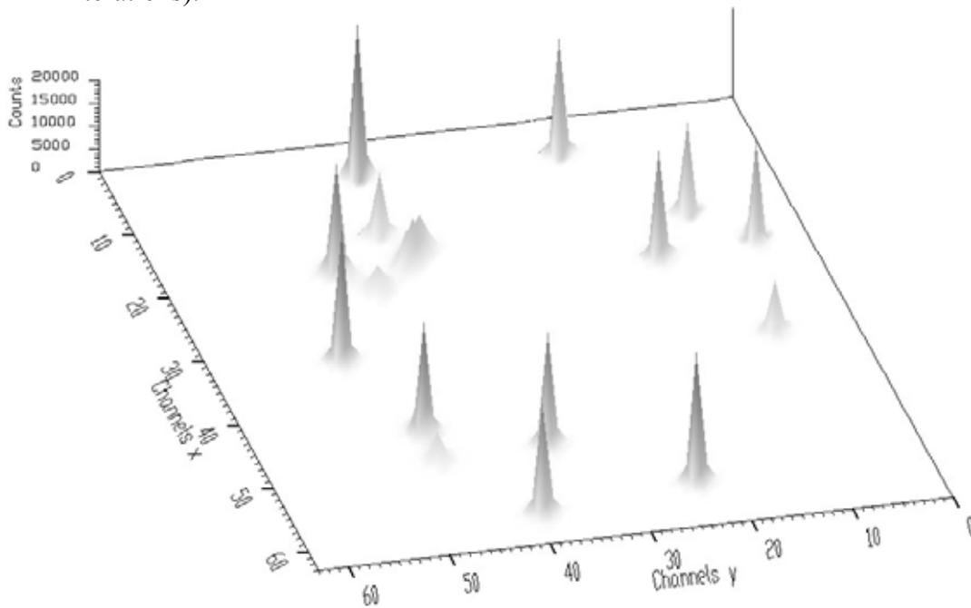
**Figure 14 Spectrum from Figure 12 after one-fold Gold deconvolution (1000 iterations)**
