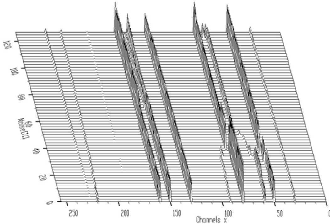
**Figure 49 Result of boosted Richardson-Lucy deconvolution for increasing level of noise**
