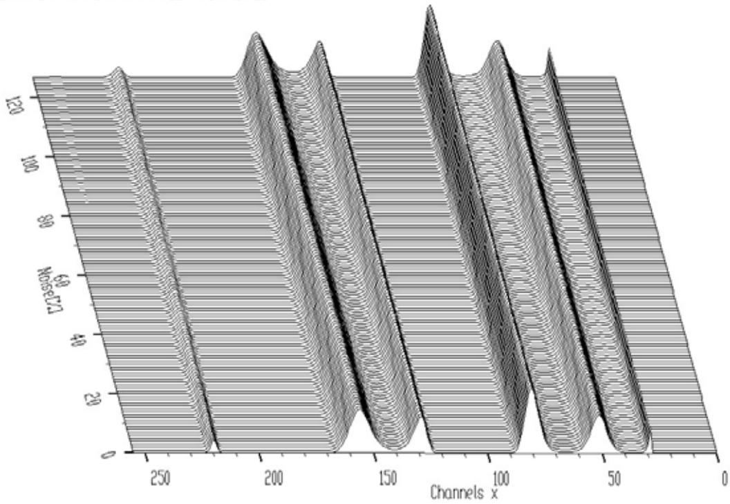
**Figure 45** Result of classic Gold deconvolution for increasing level of noise
