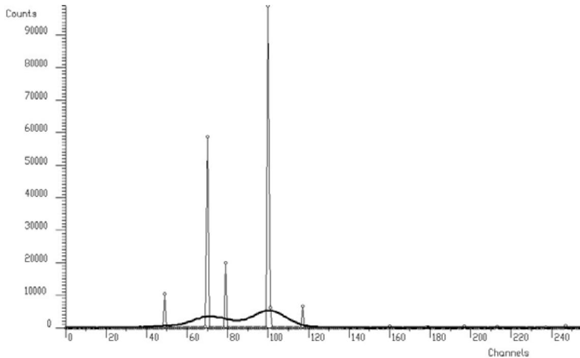
**Figure 37 Illustration of deconvolution via boosted Gold deconvolution**
