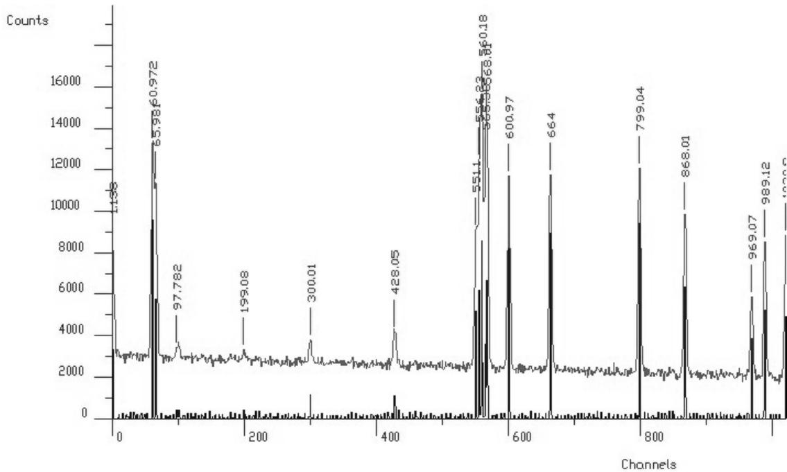
**Figure 50 Example of synthetic spectrum with doublet and multiplet and its deconvolved spectrum (in bottom part of picture)**
