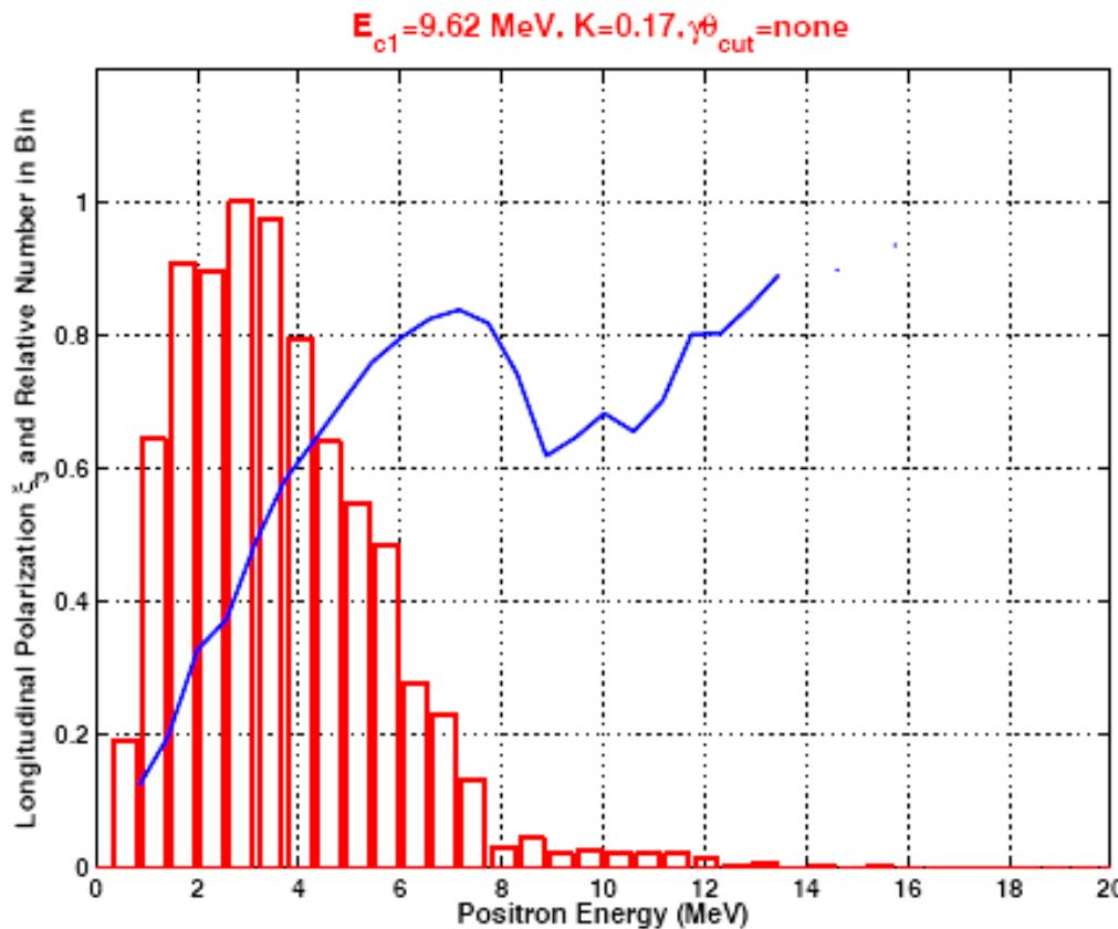
Expected positron polarization vs. positron energy
