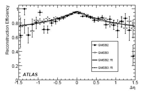
$$\begin{aligned} \Delta \eta = \eta_{true} - \eta_{rec} \\ > 90\% \text{ for } |\Delta \eta| \le 0.25 \\ \text{Falls to } \sim 75\% \text{ for } |\Delta \eta| \sim 0.5 \end{aligned}$$
