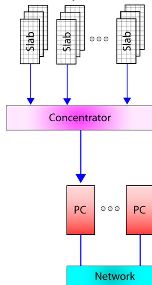
**Figure 1: The DAQ uses a classic funnel design, concentrating the data in stages before sending it to storage.**
