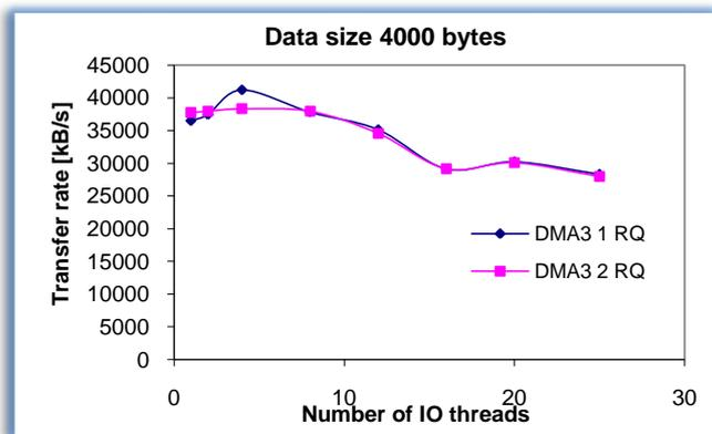
**Figure 5: Example performance of the ODR data transfer rate to disk.**
