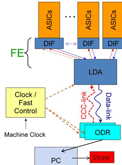
**Figure 4: Schematic of the entire DAQ showing front-end, clock and control and off-detector components. Dotted lines indicate potential synchronous, fixed latency links.**
