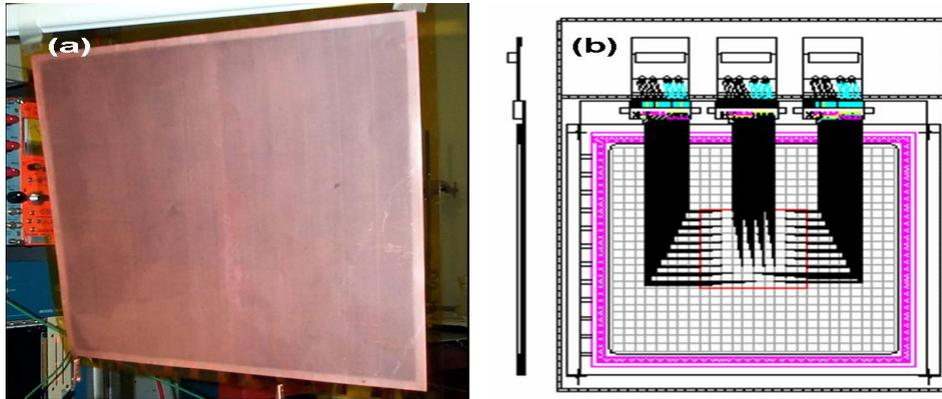
**Figure 2. (a) A photo of one of the  $30 \times 30 \text{ cm}^2$  3M GEM Foils (b) A schematic diagram of a 96 channel anode board with three 32 channel Fermilab QPA02 front end electronics**
