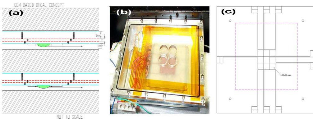
**Figure 1. (a) GEM DHCAL concept diagram (b) UTA GEM prototype chamber constructed with 10 cm×10 cm CERN GDD GEM foils (c) Prototype readout anode pad with nine 1 cm×1 cm cells**
