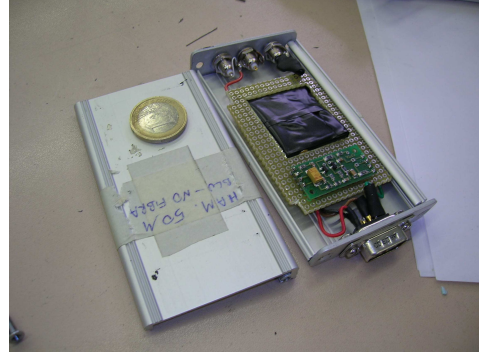
Figure 2: A counter assembly, showing the 3 by 3 \text{cm}^2 tile and the preamplifier.
