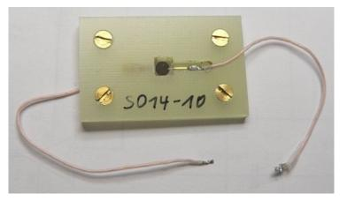
2 sensors, one is irradiated up to 5 MGy dose at the 10 MeV electron beam in 2007
