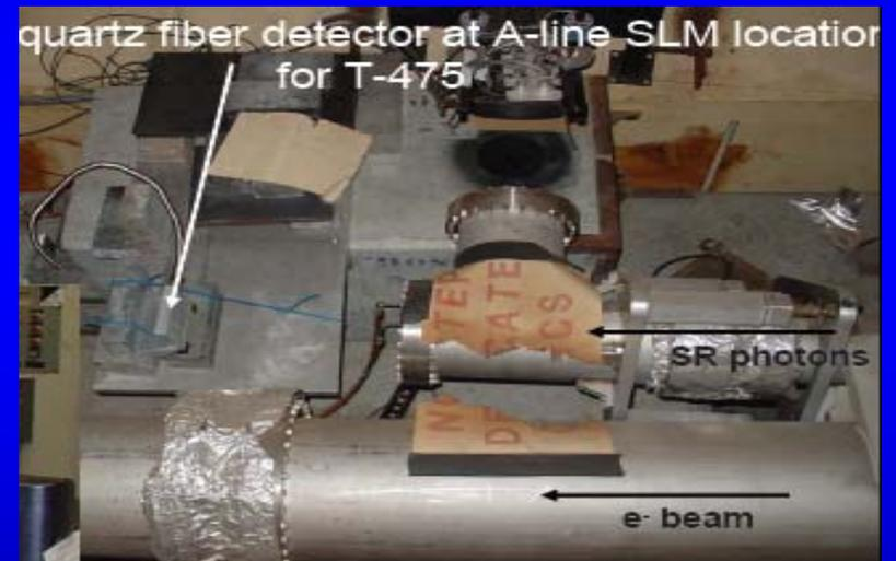
Prototype quartz fiber detector ( $8 \times 100 \mu$ m,  $8 \times 600 \mu$ m), with multi-anode PMT is installed in the A-line SLM
