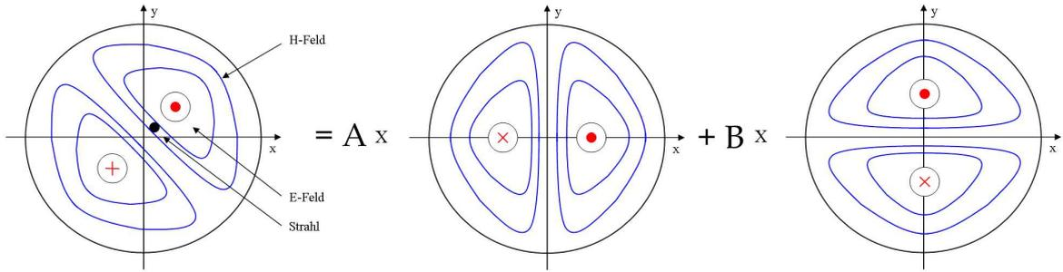
Figure 5: A generic dipole mode can be represented as a superposition of two orthogonal polarizations of the mode.
