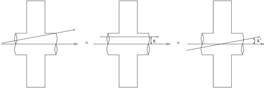
Figure 3: A generic trajectory through a cavity interpreted as a superposition of a trajectory with pure offset and a trajectory with pure inclination.
