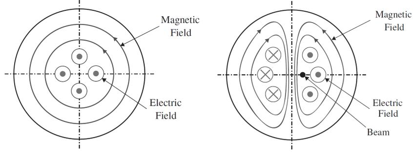
Figure 1: Left: Transverse view of the fields of the  $TM_{010}$  mode. Right: Transverse view of the fields of the  $TM_{110}$  mode. Here, the electric field has a strong dependence on the beam offset from the center of the BPM.
