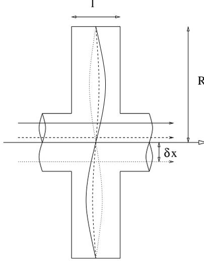
Figure 2: Schematic representation of the induced dipole mode in a cylindrical cavity. A beam with small offset (dashed line) induces a smaller signal than a beam with bigger offset (continuous line). Beams with the same offset but opposite in X induce the same signal but with opposite phases (continuous and dotted lines).
