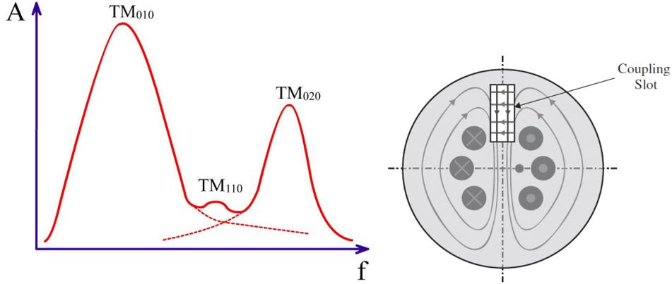
Figure 4: Left: Amplitude vs. frequency of the first two monopole modes and the first dipole mode of a cylindrical cavity with non-zero resistivity. The monopoles  $TM_{010}$  and  $TM_{020}$  surround and overlap the dipole mode  $TM_{110}$  [5]. Right: The dipole mode is selectively coupled out by means of a narrow radial slot on one face of the cavity [2].
