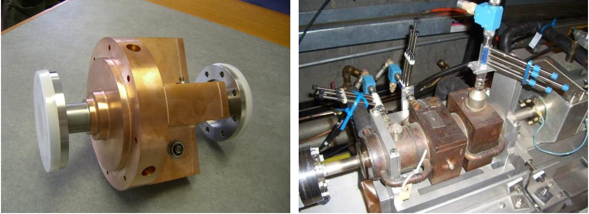
Figure 6: Left: Cylindrical cavity BPM as designed by UCL. Right: BPM 9 in End Station A. The two rectangular cavities for X- and Y-position reading and the cylindrical reference cavity are clearly seen.
