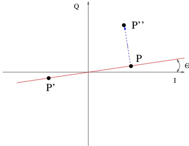
Figure 7: I-Q plot with an IQ-phase  $\Theta$ . Changing the position of the beam, the point P moves along the continuous line and changes sign when it crosses the cavity center. Changing the tilt, P moves along the dashed line, perpendicular to the continuous line.
